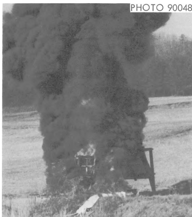
Fig. 12. IAEA 30-Min Fire Test In Progress.
