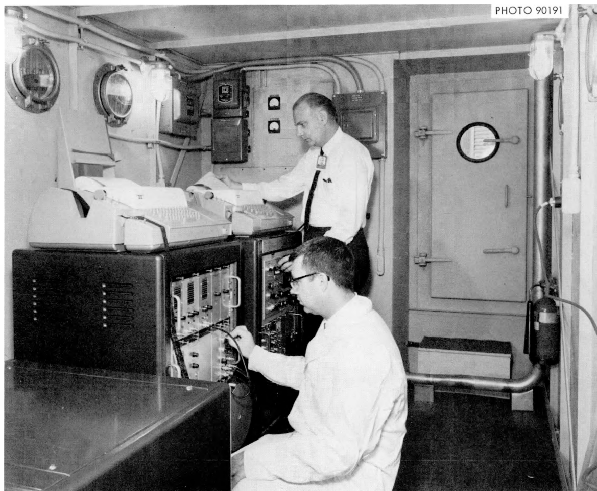
Fig. 3. Instrument Cabin for Vehicle Used to Tow Mobile Detector.
