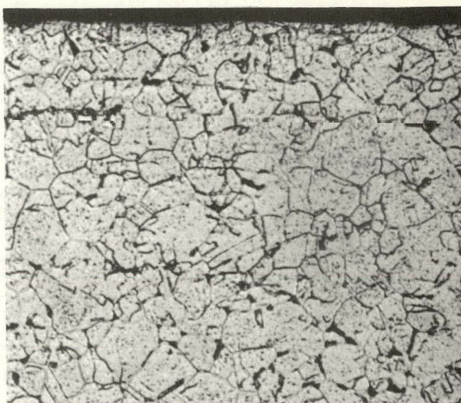
Fig. 3. Structure of Type 316 stainless steel capsule indicating no carburization during test period. Etched, 300X.
