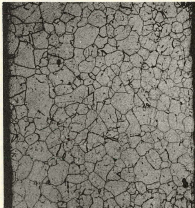
Fig. 10. Section of Type 316 stainless steel tubing from a vented (U,Pu)C fuel capsule after 900 h in 700°C sodium. 300X
