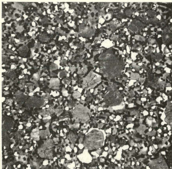
Fig. 807-1 Hyperstoichiometric UC lot 6-29-1 Before H 2 Reduction (Nitric-Lactic-Acetic etch; 380X)
