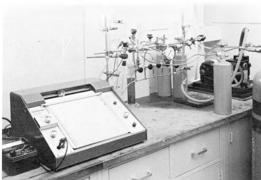
Figure 6. Apparatus for determination of trace quantities of oxygen.
