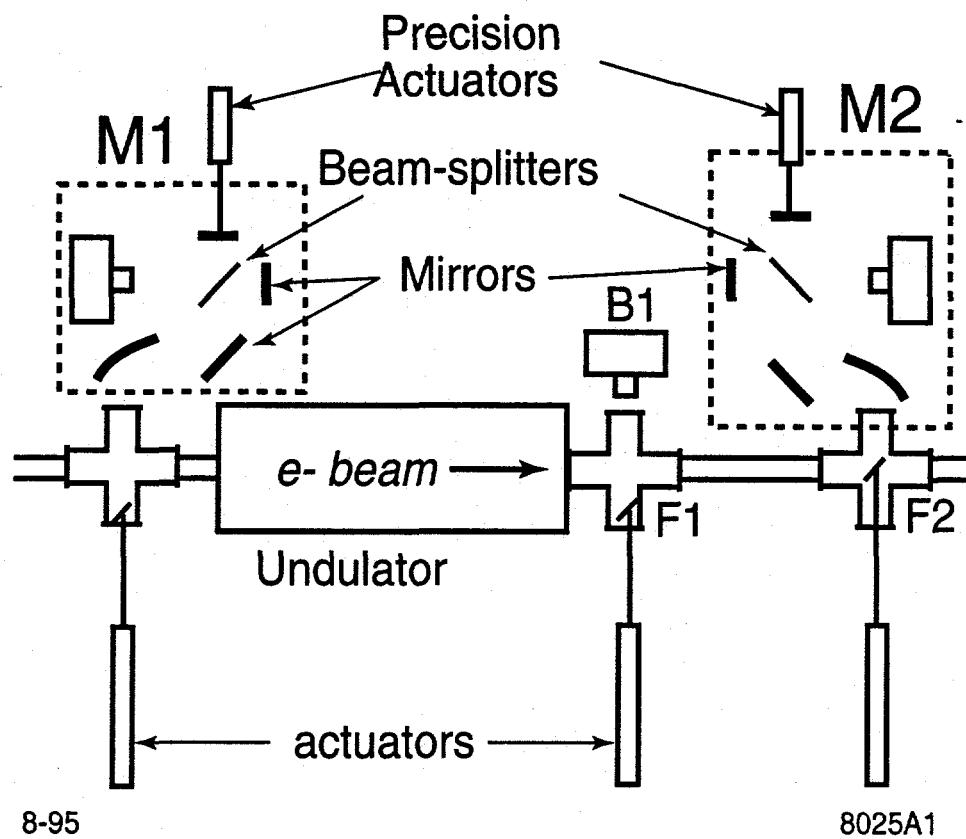
Figure 1: Experimental setup (schematically) used to measure the electron bunch length, the forward undulator radiation energy and the radiation spectrum.
