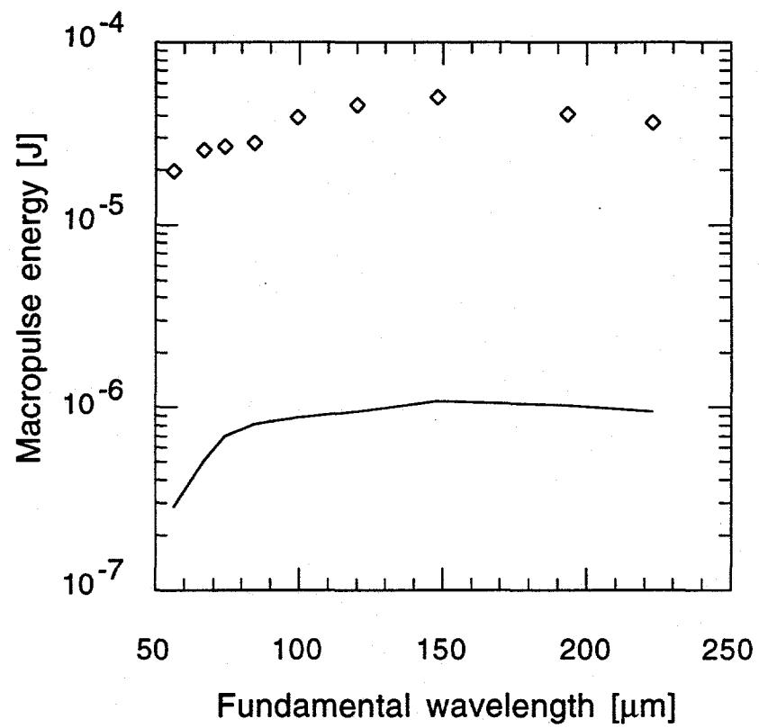
Figure 2: Radiation energy at the fundamental wavelength compared with expected spontaneous coherent undulator radiation (solid line).
