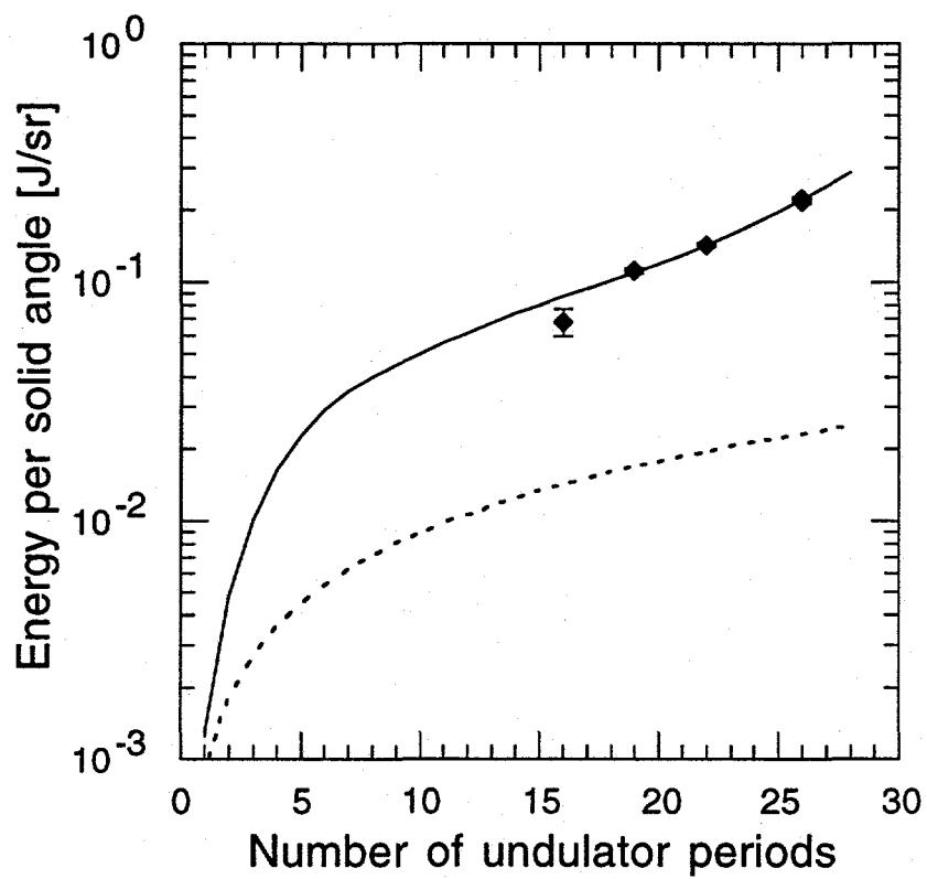
Figure 3: Measured radiation energy at  $47 \mu\text{m}$  with fit by an exponential growth theory (solid line) and compared with ordinary coherent enhancement (dashed line).
