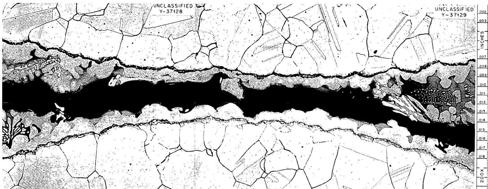
Fig. 19.20. Typical Failure in Braze Metal of Tensile-Tested Yankee Prototype Fuel Element. Etchant: 5% \text{CrO}_3 , electrolytic. Reduced 21%.
