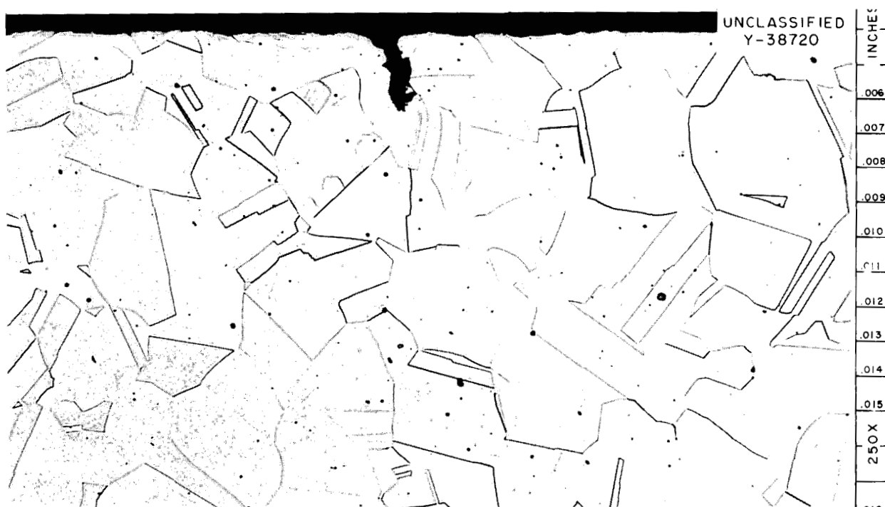
Fig. 19.17. Incipient Stress Crack in N.S. "Savannah" Piping. Etchant: aqua regia.
