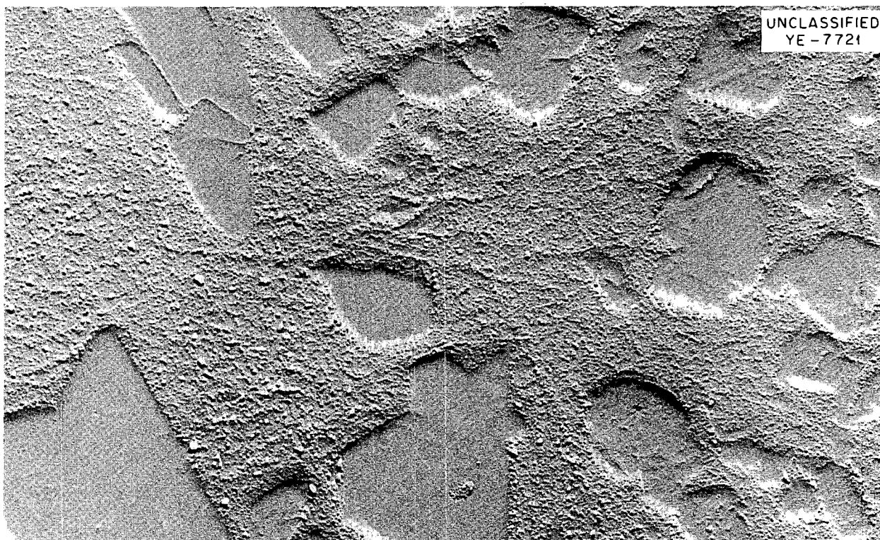
Fig. 19.2. Electron Photomicrograph of As-Polished 1-5- \mu ThO 2 Powder Particles Mounted in Glass. 13,600X.
