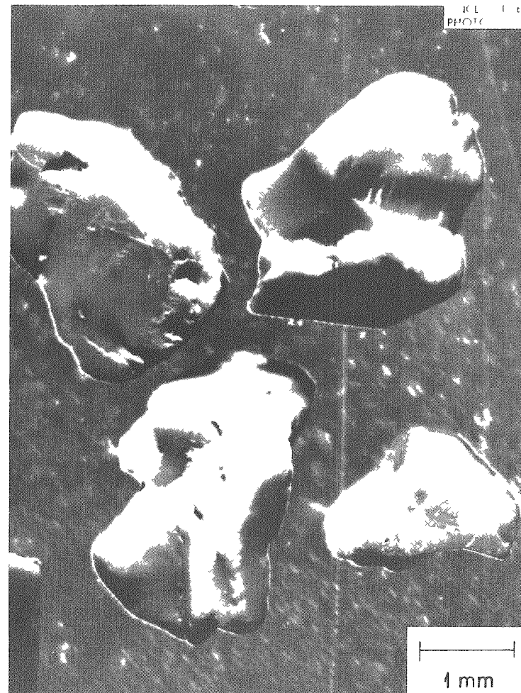
Fig. 3.8. (a) Calcined 94.8% \text{ThO}_2 -5.2% \text{UO}_{2.375} , of 1/4-in. size fraction and (b) calcined \text{ThO}_2 gel, 10-16 mesh size fraction.
