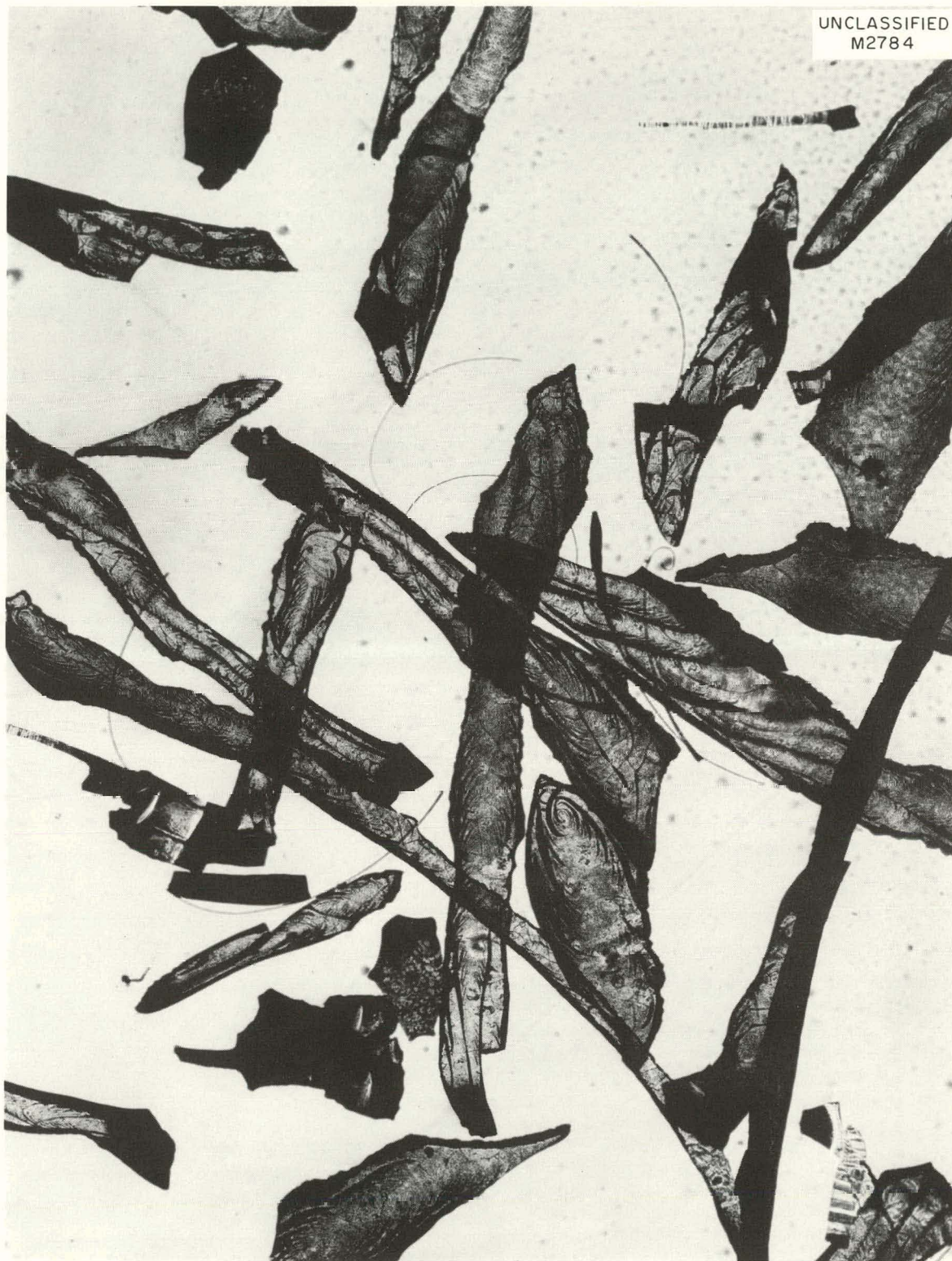
Fig. 13.2. Strained 900°C-Fired Thoria Gels from Steam-Stripped Sol Precursors Which Contained Excessive Nitrate. 18X.
