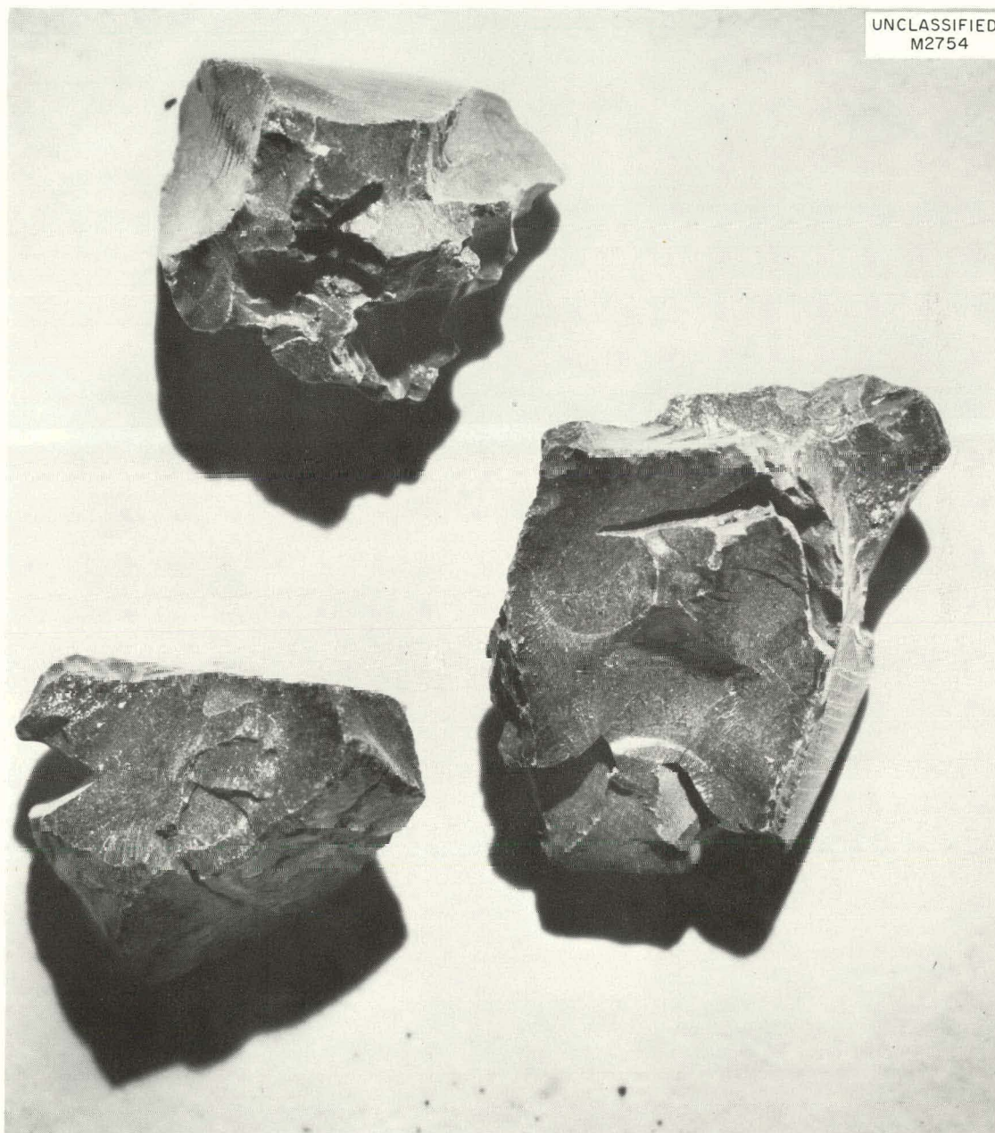
Fig. 13.3. Thorium-5 wt % Uranium Fragments Prepared from Oxalate-Derived Thoria Sols Before Grinding in Spouted Bed. 12X.
