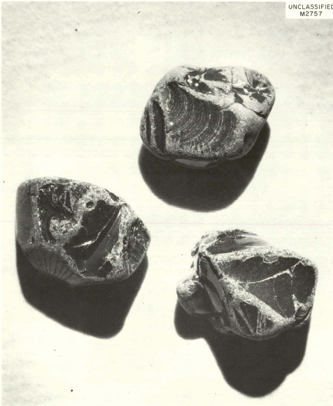
Fig. 13.4. Thorium-5 wt % Uranium Fragments Prepared from Oxalate-Derived Thoria Sols After Grinding 6 hr in Spouted Bed. 12X.
