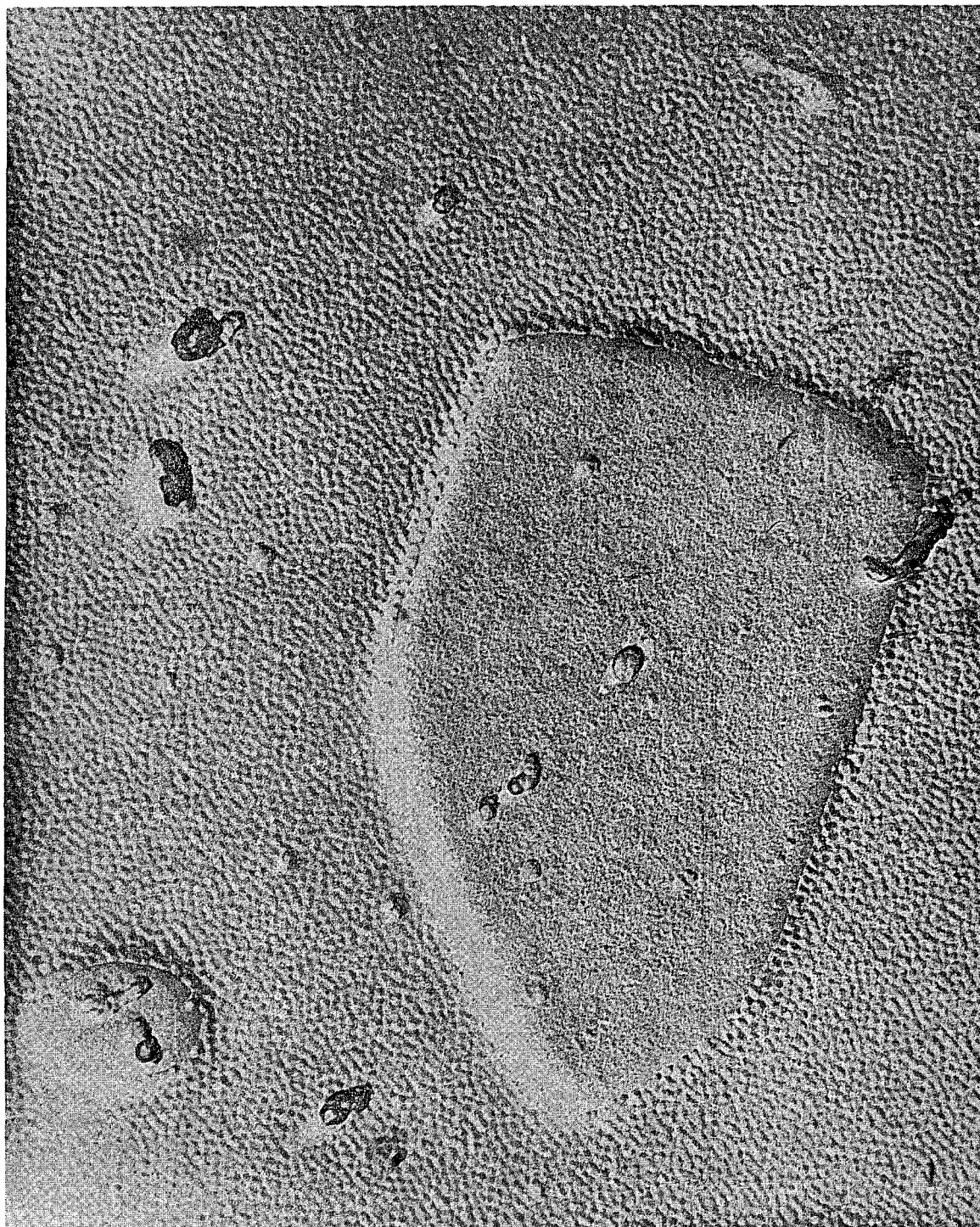
Fig. 5. "Delta"-Phase Particles in Hot-Worked, Alloyed Dingot Uranium (300 PPM Fe - 200 PPM Si) Alpha Annealed for 256 Hours at 1160°F.
