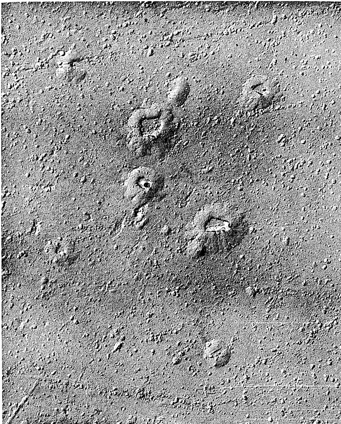
Fig. 1. "Delta"-Phase Particles in Hot-Worked, Alloyed Dingo Uranium (300 PPM Fe - 200 PPM Si) Alpha Annealed for 6 Hours at 1160°F.
