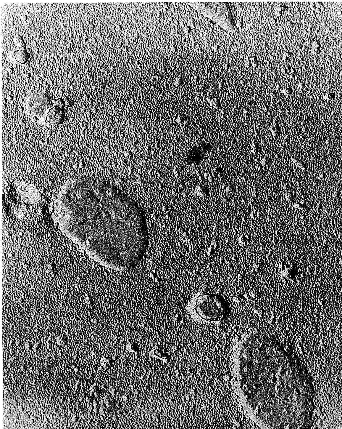
Fig. 3. "Delta"-Phase Particles in Hot-Worked, Alloyed Dingot Uranium (300 PPM Fe - 200 PPM Si) Alpha Annealed for 112 Hours at 1160°F.
