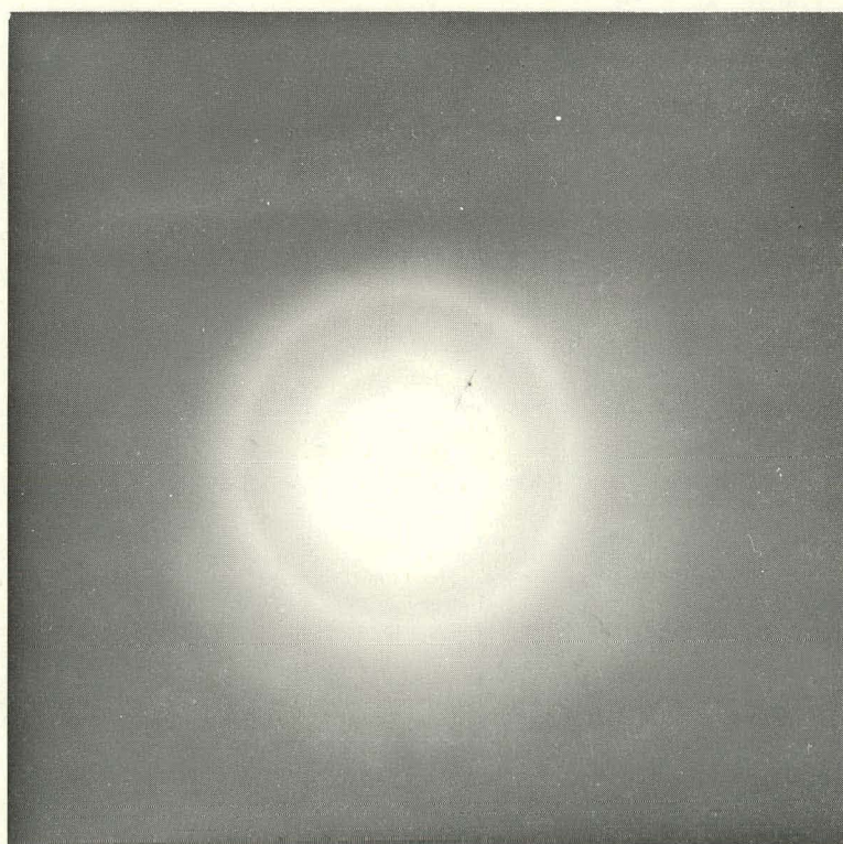
Fig. 12. Electron Diffraction Pattern of Amorphous (to X-ray) Alumina
