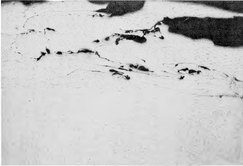
Figure 103. Photomicrograph of RPI hot-ductility bar of high-manganese Type 347 weld metal illustrating the intergranular nature of failure and the continuous intergranular precipitate. This specimen was tested at 2300°F on cooling from 2400°F. X50
