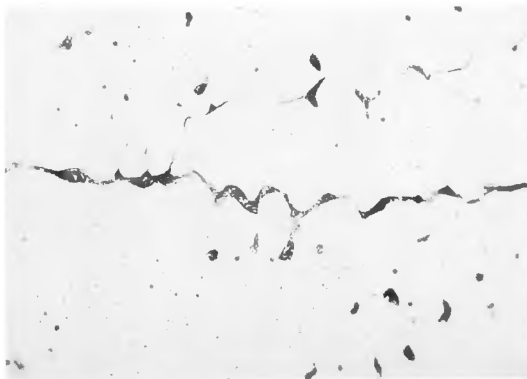
Figure 80. As welded microstructure of Composition A deposit. Ferrite is observed in a matrix of austenite.
