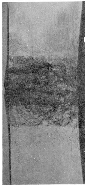
37% Elongation Bend Angle 80° Specimen H8
