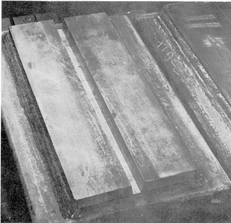
Figure 15. Butt weld test plates before welding.
