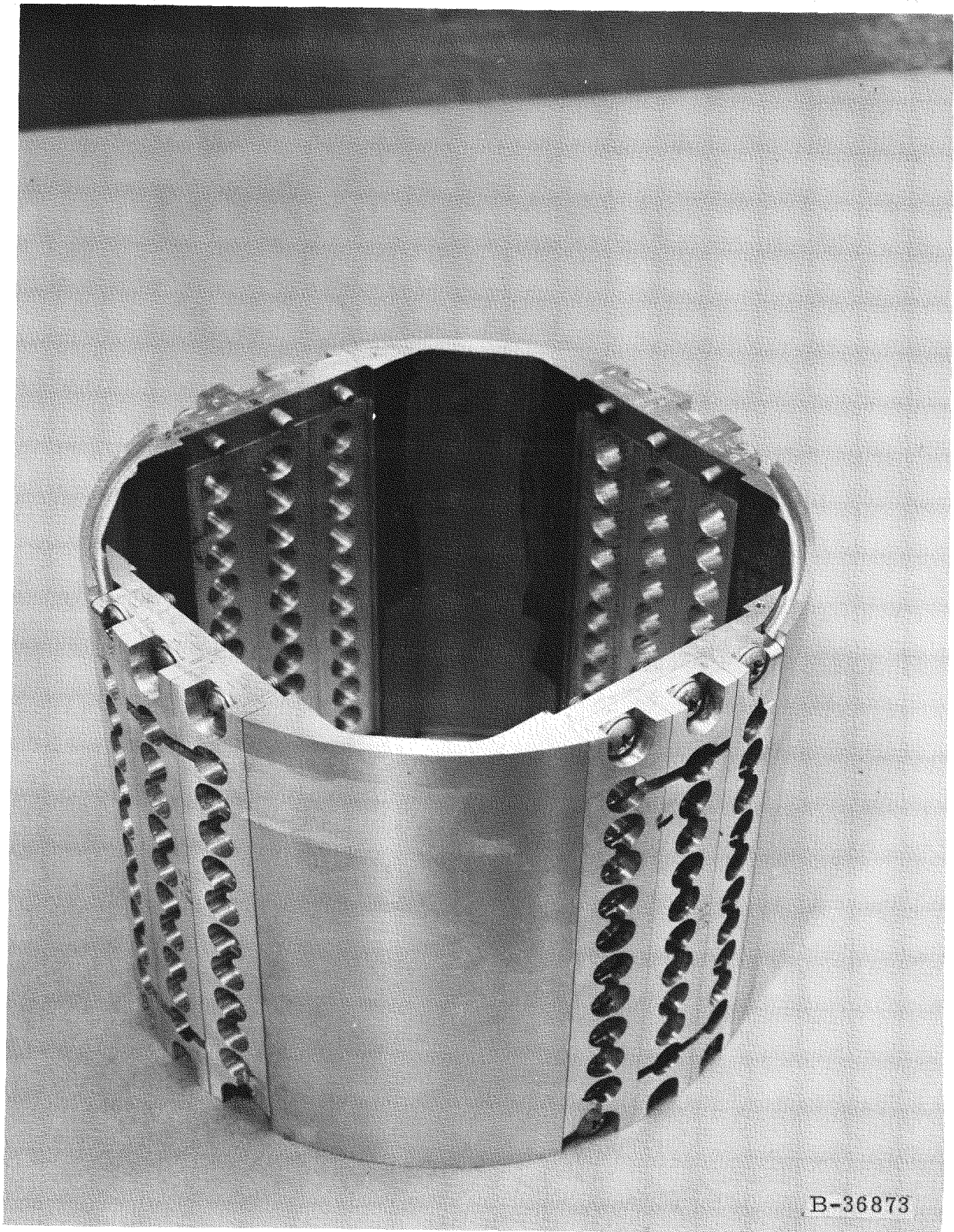
Fig. A-3. SNAP 7A and 7C Heat Sink After Turning
