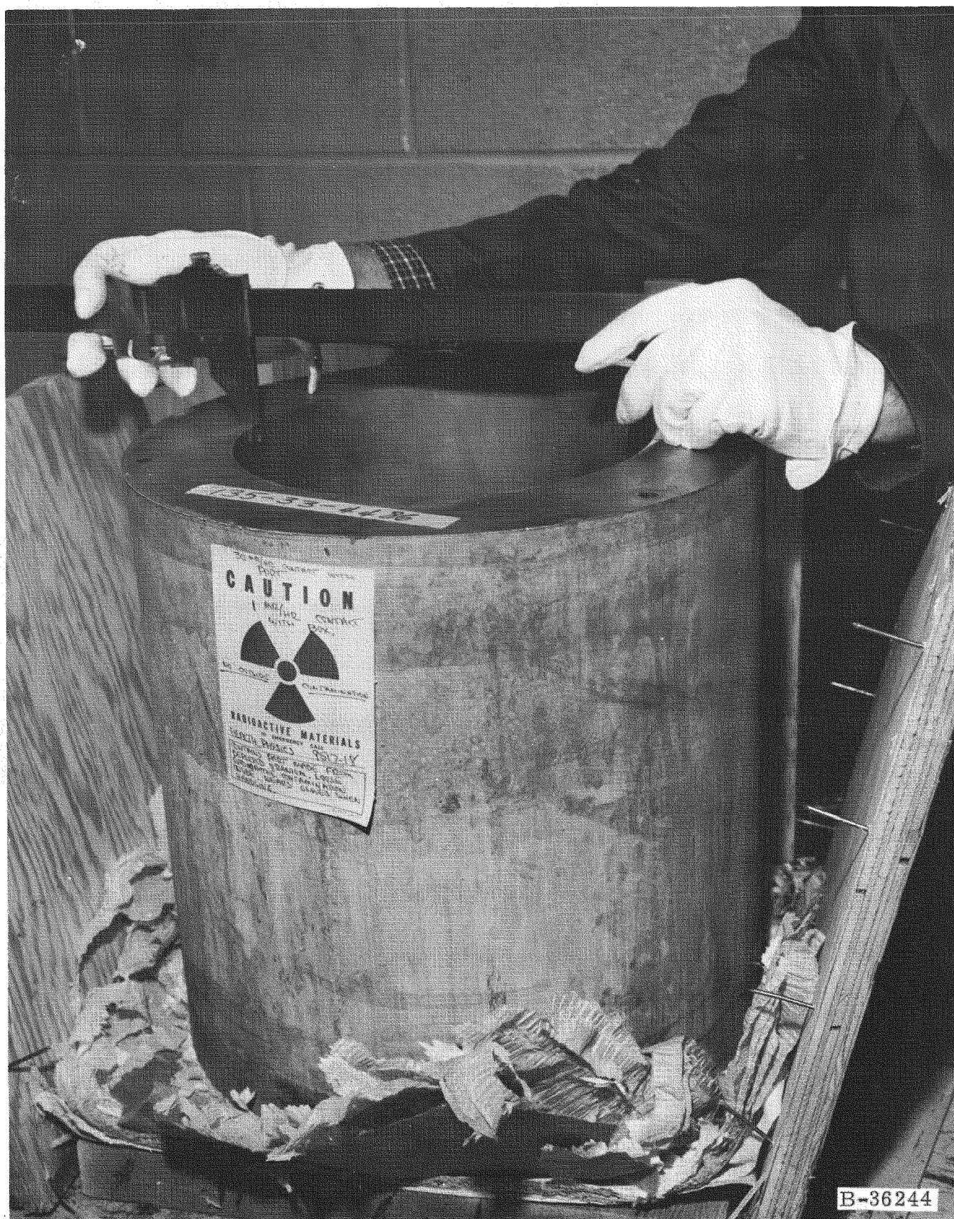
Fig. A-8. SNAP 7A and 7C--Depleted Uranium for Use in Biological Shield
