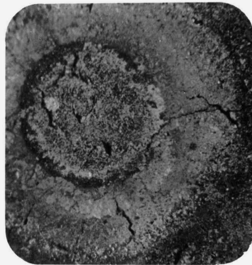
Figure 5 A pellet face from specimen AHL with concentric colouration rings on the surface. Note the porous center of the \text{UO}_2 pellet.
