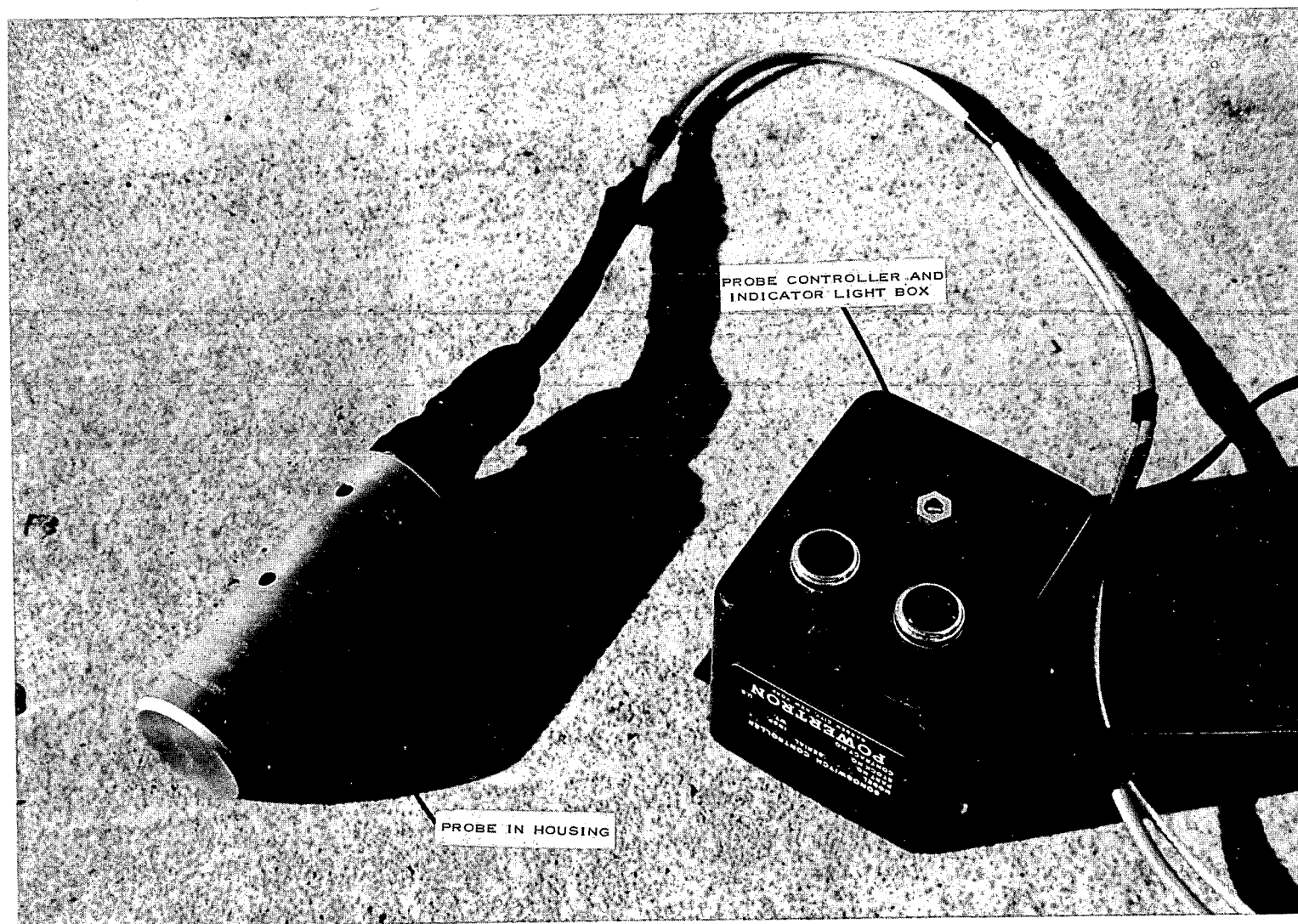
Figure 26 Ultrasonic Probe and Housing for Water Detection
