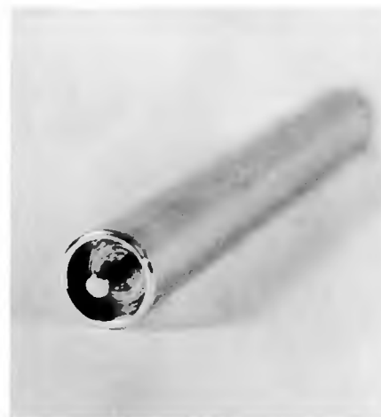
Fig. I-2. Typical Specimen Tube End Closure ( \sim 2X )
