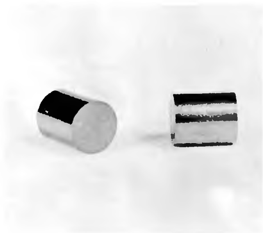
Fig. I-1. Enriched \text{UO}_2 Pellets ( \sim 2X )
