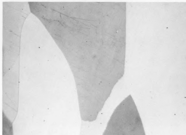
FIGURE 20. EVIDENCE OF COMPLETE DEPLETION OF UC_2 SECOND PHASE NEAR SURFACE OF URANIUM-5.0 w/o CARBON SPECIMEN IRRADIATED AT 580 TO 770 C TO A URANIUM BURNUP OF ABOUT 0.48 a/o
