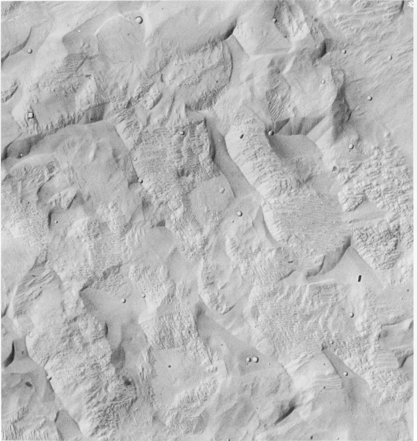
FIGURE 25. STRUCTURE OF URANIUM-6.7 w/o CARBON ALLOY ETCHED HEAVILY BY VACUUM-CATHODIC TECHNIQUES
