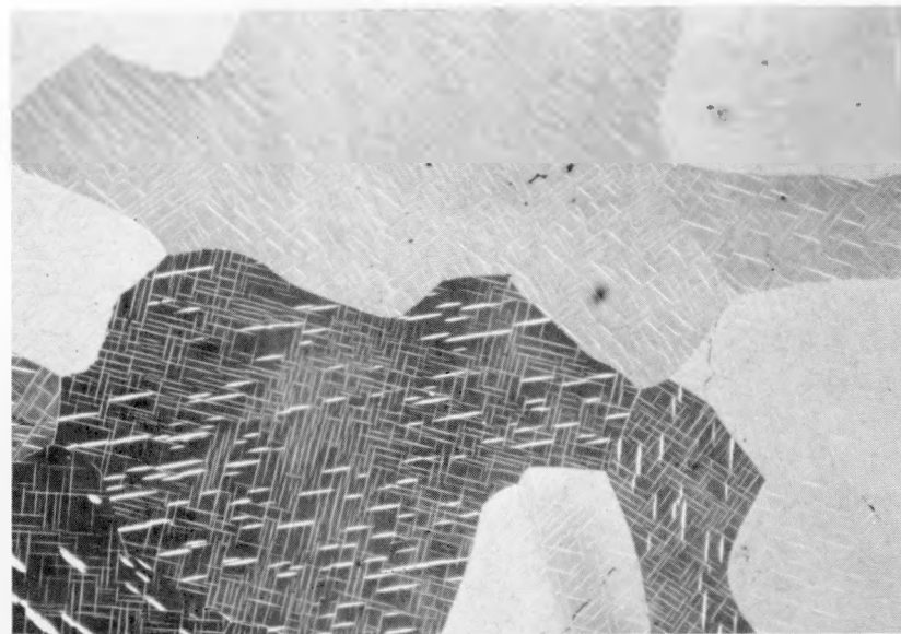
FIGURE 14. TYPICAL MICROSTRUCTURE OF URANIUM-5.0 w/o CARBON SPECIMEN AFTER IRRADIATION AT 150 C TO A URANIUM BURNUP OF 0.15 a/o
