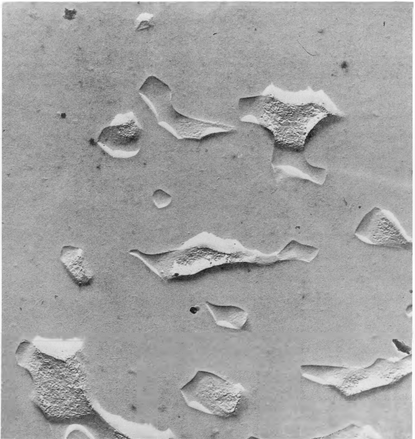
FIGURE 24. STRUCTURE OF URANIUM-6.7 w/o CARBON ALLOY CHEMICALLY ETCHED PRIOR TO IRRADIATION
