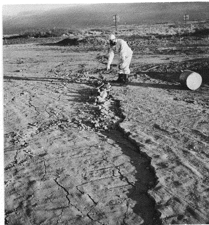
Figure 4.4 Concentric Fault Located 40 Meters Southwest of Surface Ground Zero.
