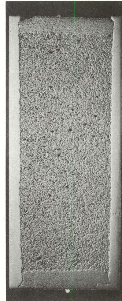
Fig. 4.3. Pressed pellets in aluminum cups. (a) 15-mil-wall cup, longitudinal section; (b) 5-mil-wall cup; (c) powder plugs at both ends.
