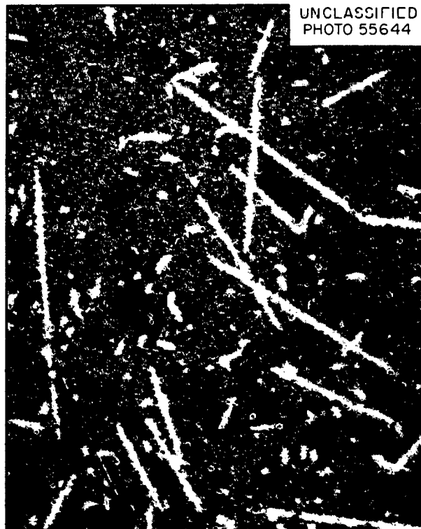
Fig. 13.1. Fission-Fragment Tracks in 25-A-thick Palladium Film. 50,000X.
