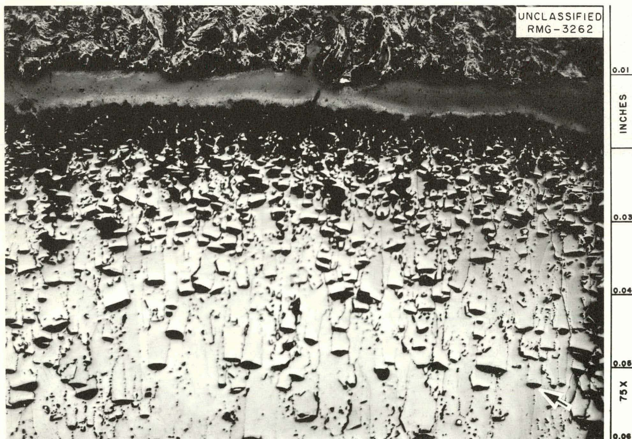
Fig. 21.16. Voids in \text{UO}_2 Deposited in Ends of Cylinder.
