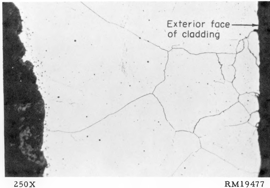
FIGURE 15. PRESSURE-BONDED TYPE 304L STAINLESS STEEL AFTER CORROSION TESTING FOR 48 HR IN 750 F STEAM
