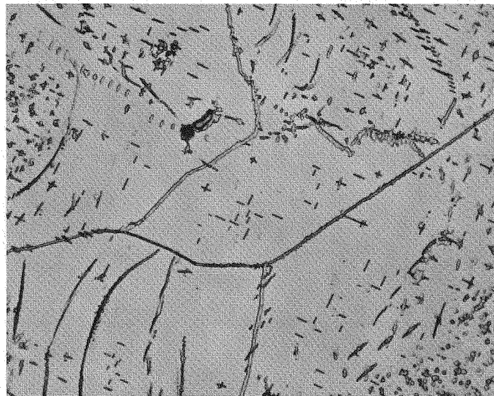
Figure 5. Alloy 16M annealed one day at 1110°C, then twenty-four hours at 550°C, and air cooled. (500X)
