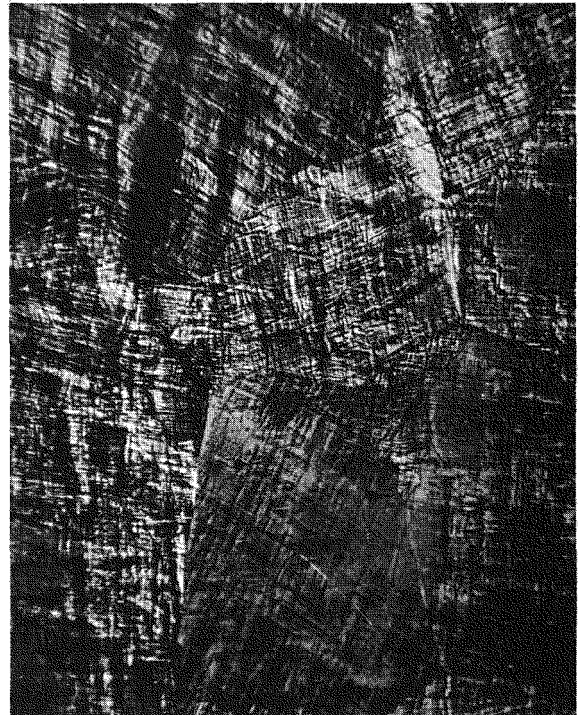
Figure 8. Alloy 16M annealed four days at 1110°C, then seventy-two hours at 550°C, and air cooled. Photographed in bright field to reveal alpha phase and in polarized light to reveal gamma prime phase. ((500X BF and 100X PL)
