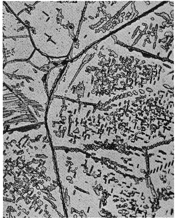
Figure 7. Alloy 16M annealed six days at 1110°C, then forty-eight hours at 550°C, and air cooled. (500X)
