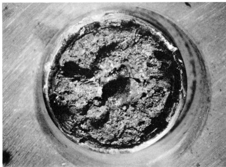
Figure 22. Fracture Surface of Bottom Pellet in Molybdenum-fibered, Lead-bonded Specimen ANL-35-18, Showing Mixture of Lead and Oxide after a Burnup of 29,700 MWD/T and an Integral kd\theta Value of 122 w/cm.
