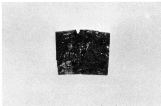
Figure 10. Specimen ANL-35-3 after a Burnup of 9200 MWD/T and an Integral kd_0 Value of 51 w/cm, Showing Typical Damage Received by Unclad, Niobium-fibered Pellets.
