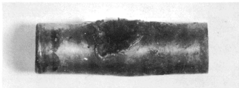
Figure 6. Helium-bonded, Molybdenum-fibered Specimen ANL-35-36 after a Burnup of 17,400 MWD/T and an Integral kd\theta Value of 103 w/cm Showing Cladding Burnout and Exposed Fuel.
