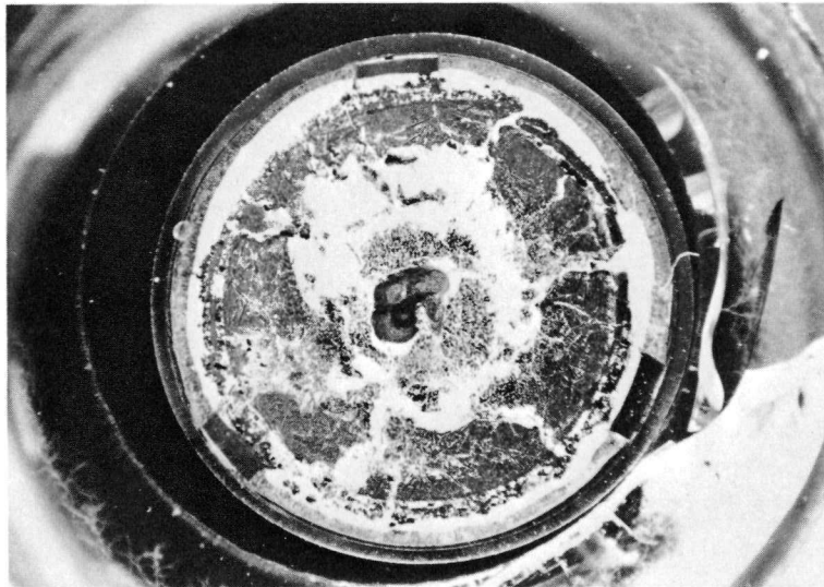
Figure 39. Polished Section of Molybdenum-fibered Specimen ANL-35-18 after 29,700 MWD/T at an Integral kd\theta Value of 122 w/cm. White Areas Are Lead. Note the Reduction in Size of the Three Zircaloy-2 Ribs.
