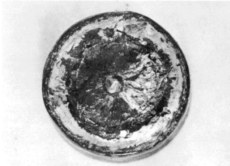
Figure 17. Fracture Surface of Bottom Pellet in Unfibred, Lead-bonded Specimen ANL-35-28, Showing Radial Columnar Grains and a Small Central Void Filled with Lead after a Burnup of 11,300 MWD/T and an Integral kd\theta Value of 68 w/cm.
