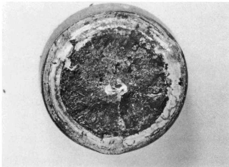
Figure 20. Fracture Surface of Bottom Pellet in Molybdenum-fibered, Lead-bonded Specimen ANL-35-26, Showing Area Just Below Small Central Void after a Burnup of 17,000 MWD/T and an Integral kd\theta Value of 96 w/cm.
