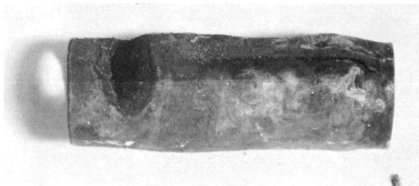
Figure 2. Lead-bonded, Molybdenum-fibered Specimen ANL-35-17 after a Burnup of 31,100 MWD/T and an Integral kd\theta Value of 129 w/cm Showing Cladding Burnout and Longitudinal Crack.
