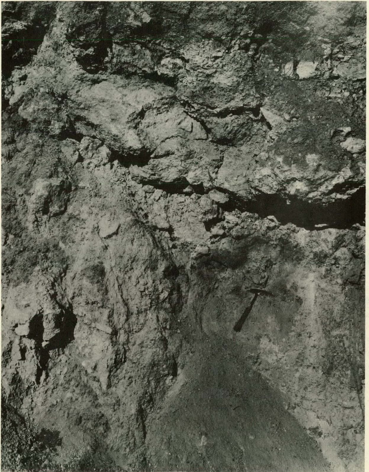
Fig. 4. Rock exposure on side of excavation in vesicular facies of Ribbon Cliff formation at Palanquin site.
