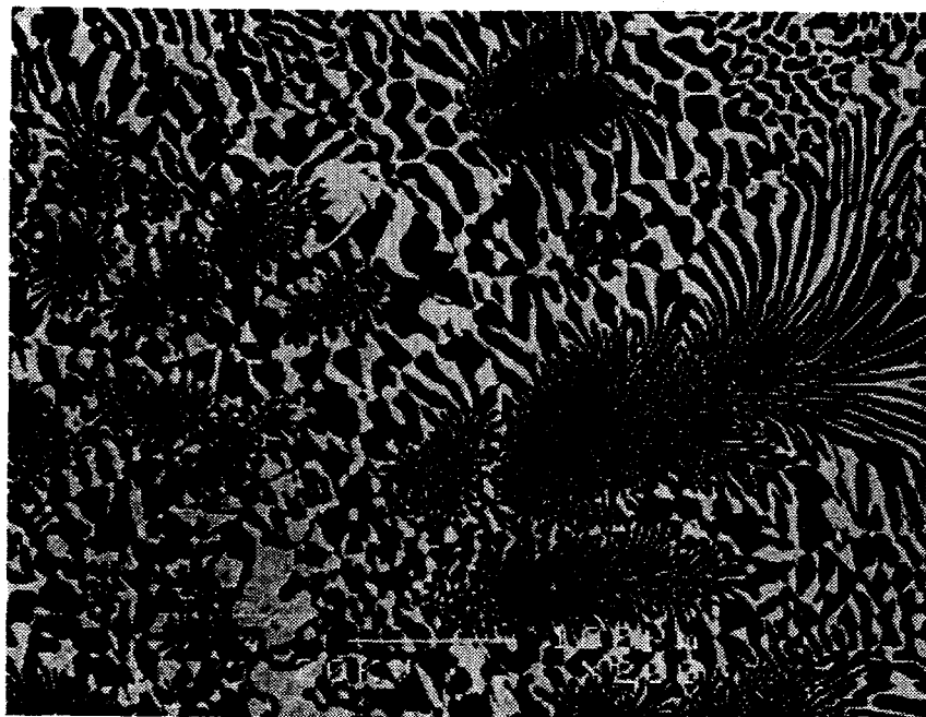
Fig. 1. Typical microstructure of as-cast SS-15Zr alloy. The dark phase is \alpha -SS, the bright phase \text{Zr}(\text{Fe}, \text{Cr}, \text{Ni})_{2+x} .
