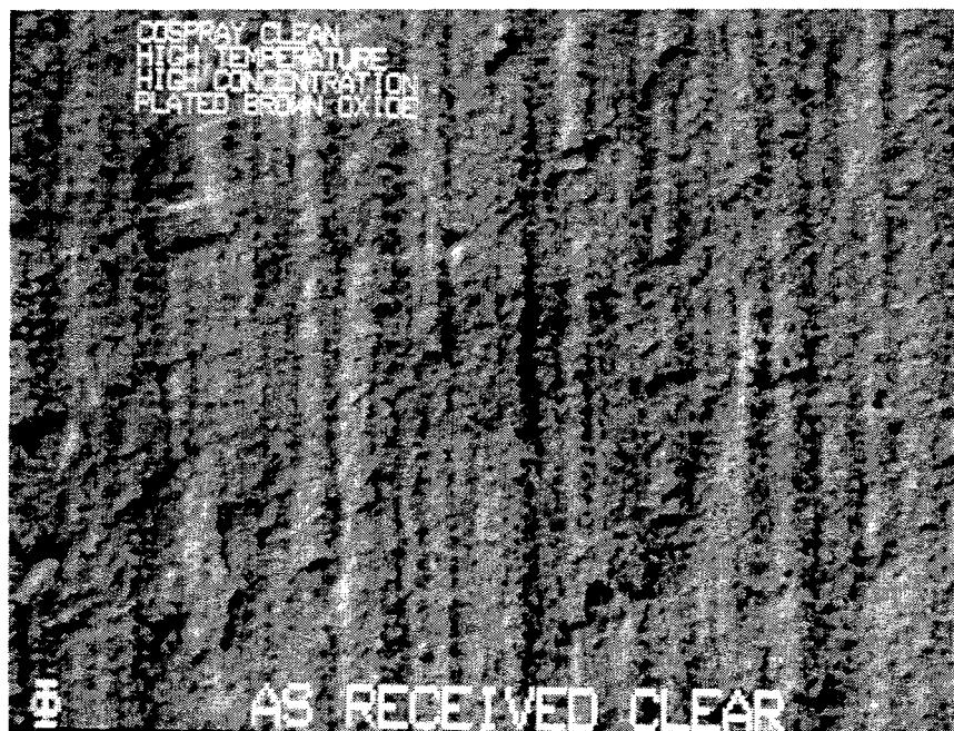
a. COSPRAY-CLEANED COPPER WITH PLATED BROWN OXIDE. (COPPER WAS CLEAR PRIOR TO CLEANING.)
