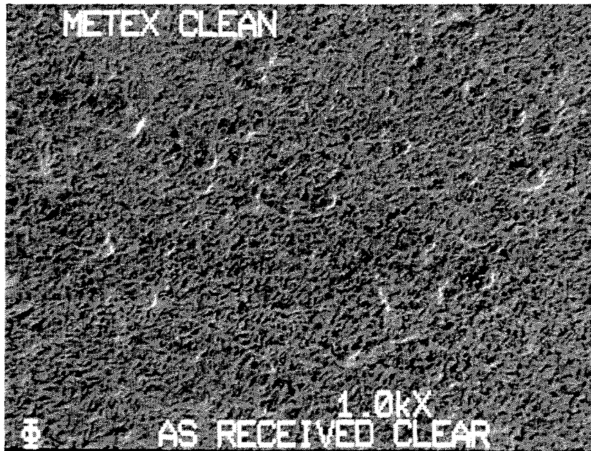
a. CLEAR COPPER, METEX CLEANED
