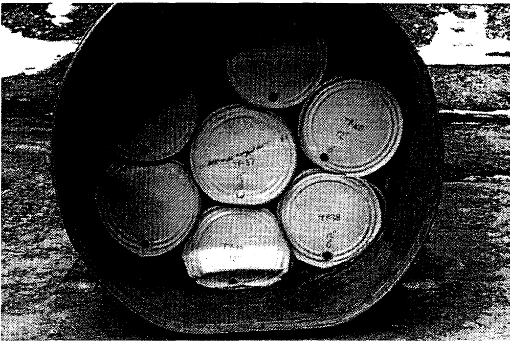
Figure 10: Damage to the seven-pack of 12" Pipe Overpack Containers during the ICV drop test.
