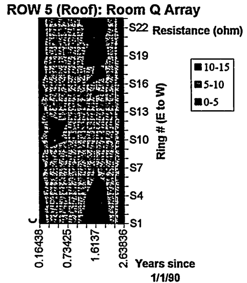
Figure 3d: Change in resistance with time along Room Q roof
