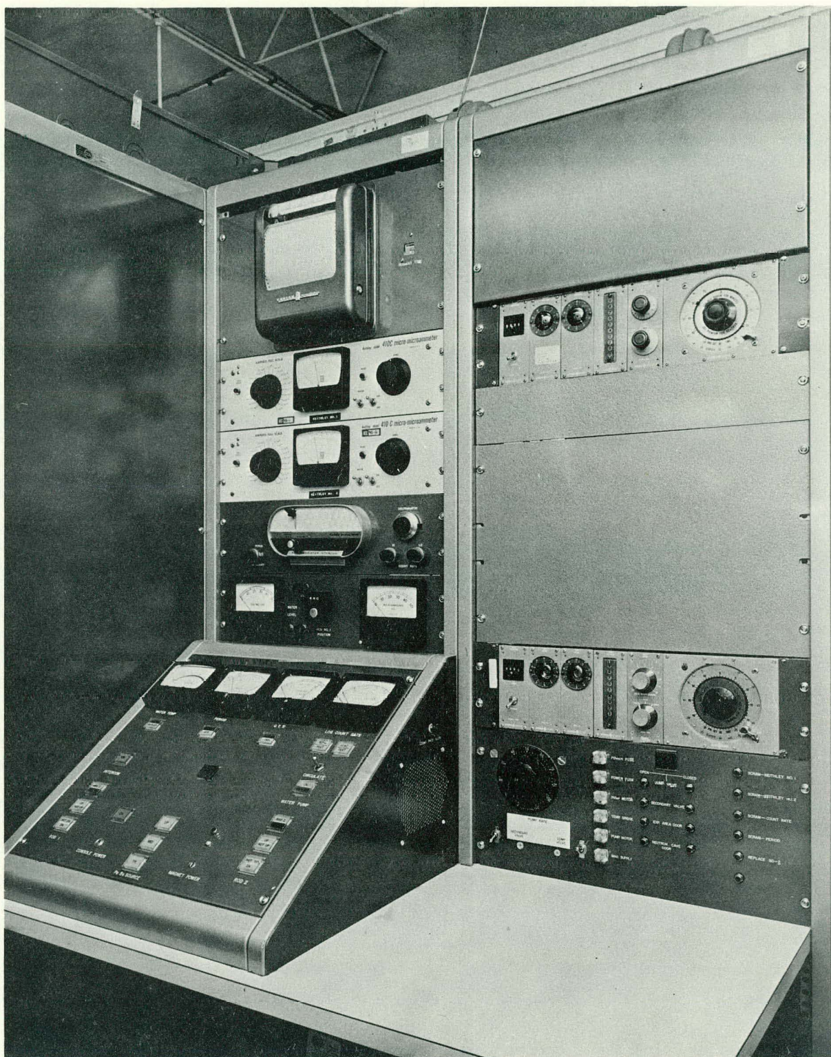
Fig. 3--Control console for the subcritical assembly
