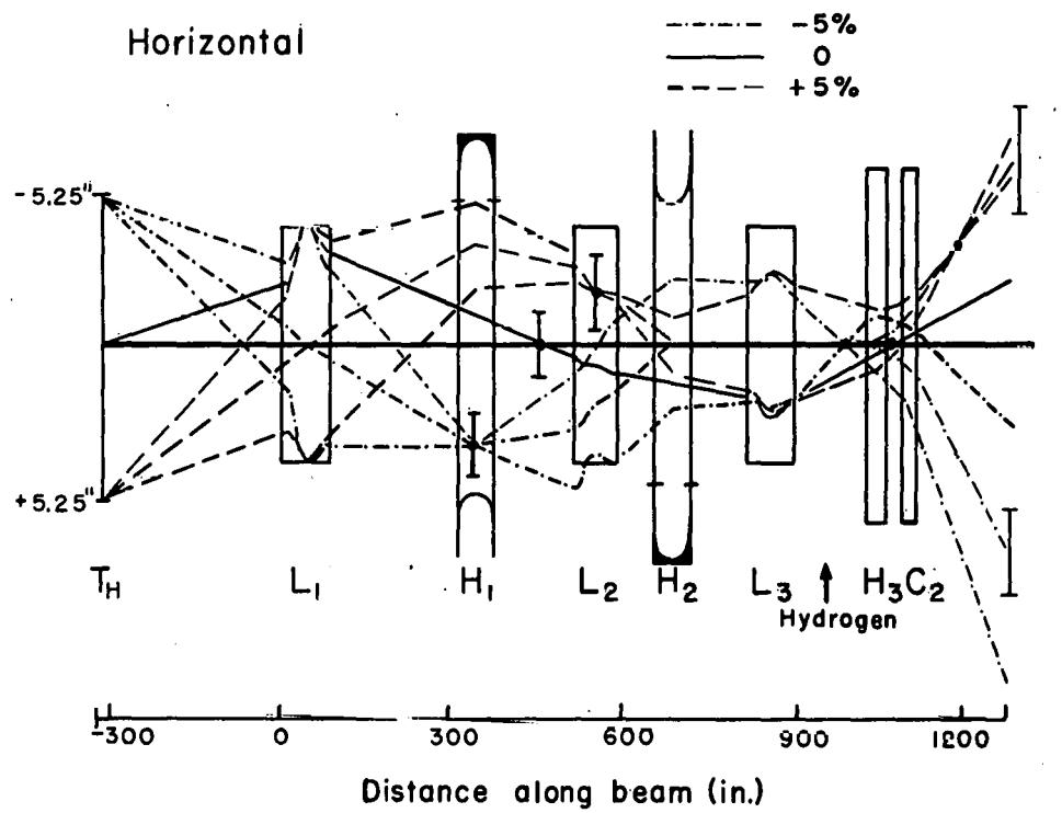
Fig. 2B. Schematic diagram of beam. Horizontal plane.  $T_H$  is the virtual target in the horizontal plane.
