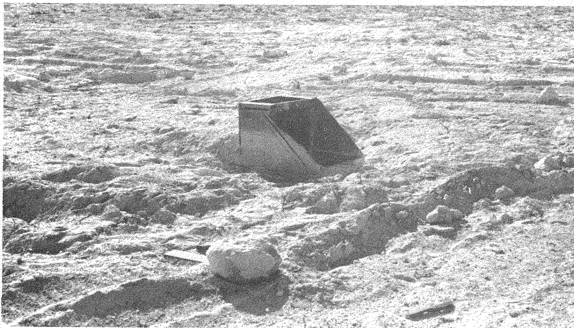
Fig. 5.3 Shelter A-6 After Shot Charlie (lightened-frame below-grade)
