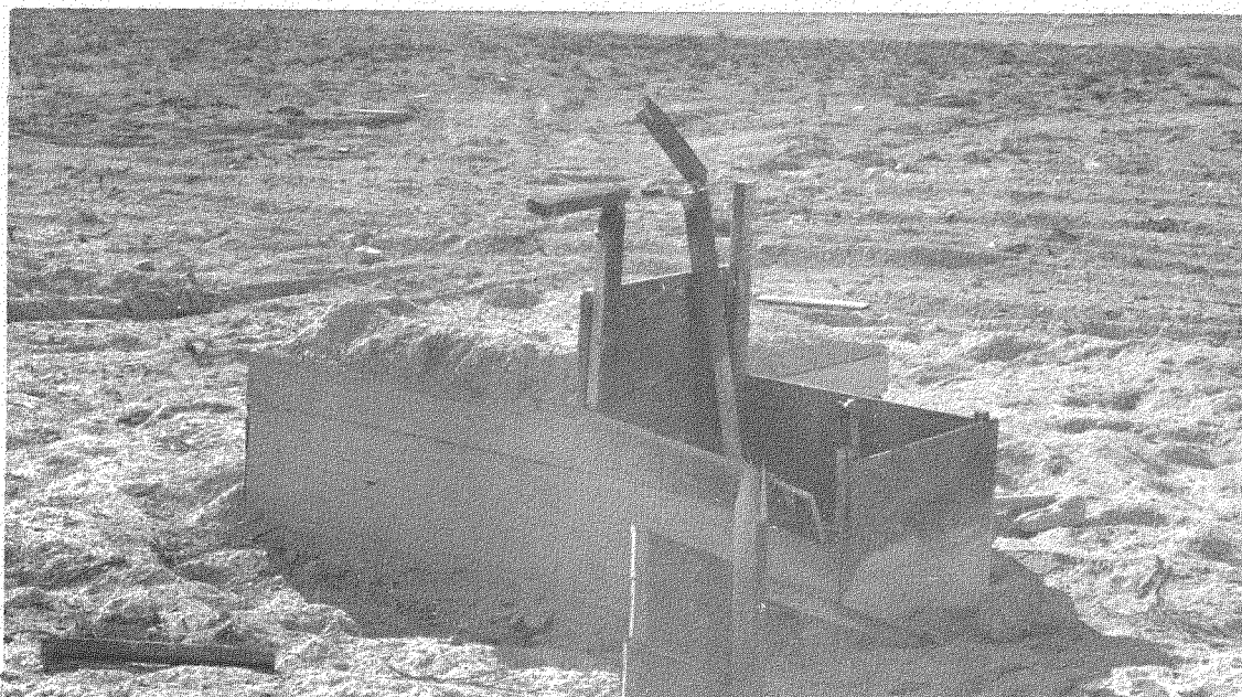
Fig. 5.4 Shelter A-9 After Shot Charlie (partly above-grade lightened-frame)
