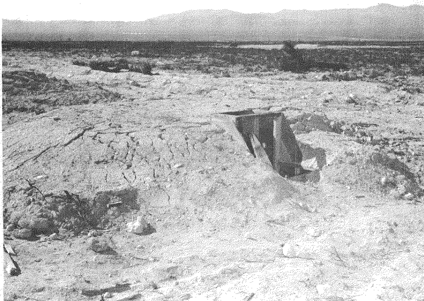
Fig. 4.2 Shelter A-2 After Shot Baker (covered- trench below-grade)
