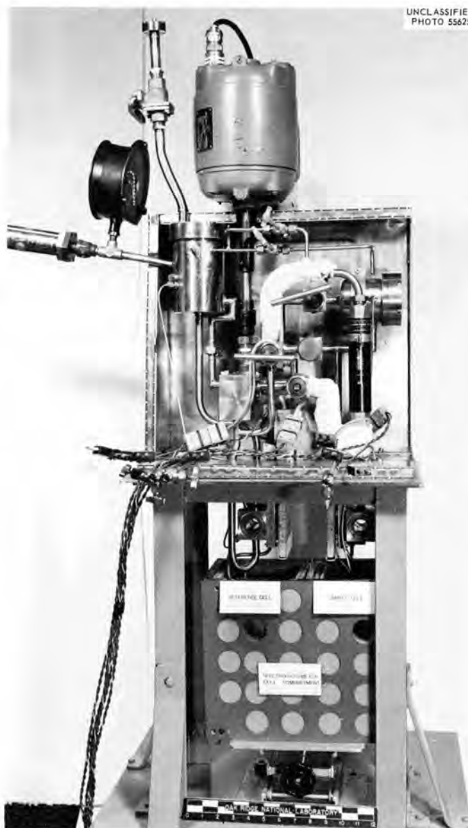
Fig. 3.2. Closeup View of the Circulating Loop System of the Cary Model 14PM Spectrophotometer, Together with Its Companion Spectrophotometer Cell Compartment.
