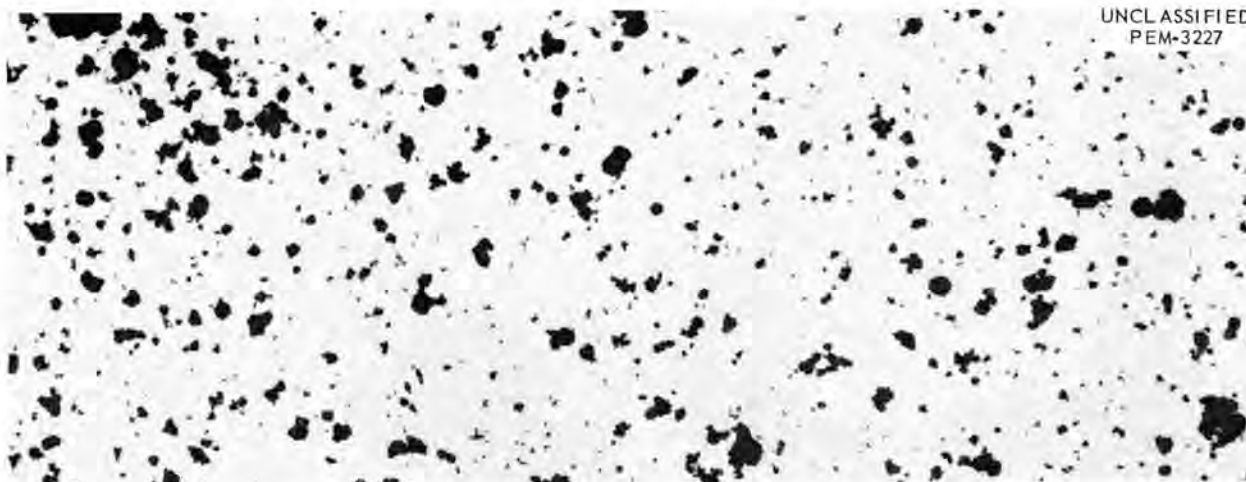
Fig. 7.1. Electron Micrograph of Particles of \text{ThO}_2 Taken from an In-Pile-Loop Sample. 8000X.
