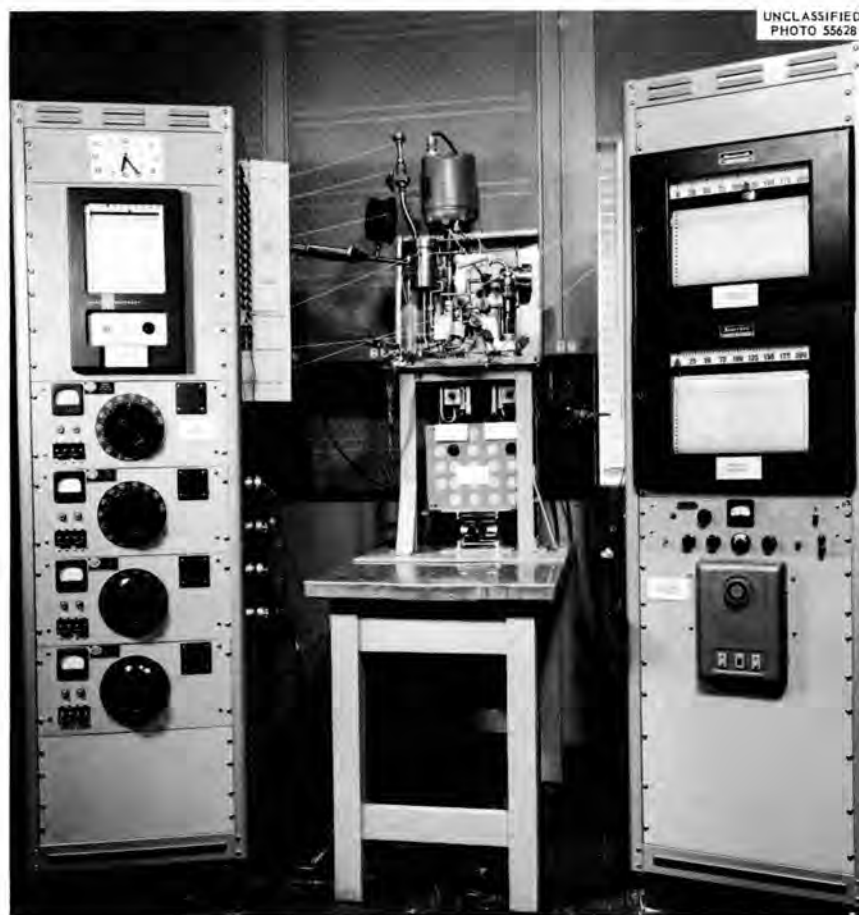
Fig. 3.1. Circulating Loop System for the Cary Model 14PM Spectrophotometer with Related Control Instrumentation. (Loop is removed from the spectrophotometer system.)
