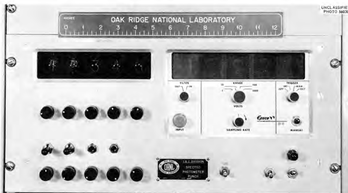
Fig. 3.4. Closeup View of the Main Control Panel of the Automatic, Digital, Data-Output System for the Cary Model 14PM Spectrophotometer.
