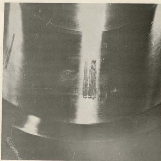
Figure 5. Test 2 - 17-4PH stainless steel nozzle (top) and 304 stainless steel sleeve (bottom) after galling test with 165-lb horizontal load. (NP Photo 18A-12, -13, -15, -16)
