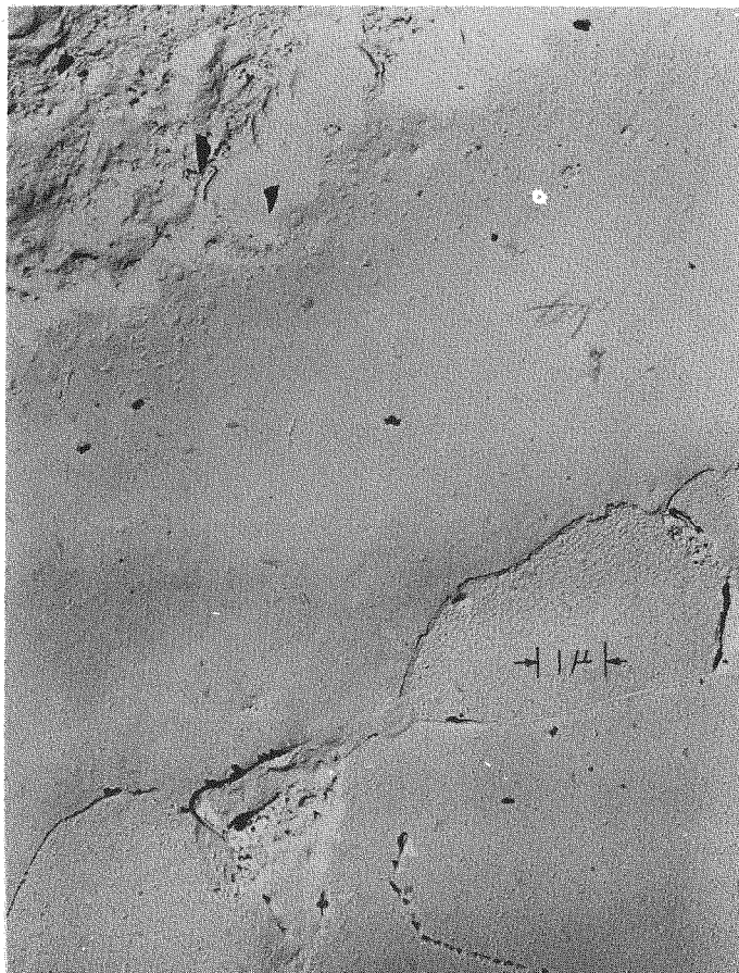
Figure 6. Electron micrograph of \text{Al}_2\text{O}_3 -Coated \text{UO}_2 (Lot 4E). (N-79982)
