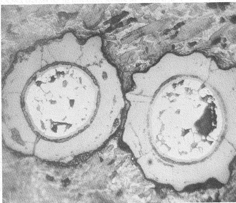
Figure 5. Typical Failed Particles from Lot 4E After Irradiation to 6 per cent Burn-Up of U^{235} in 160 Days at 700°C.
