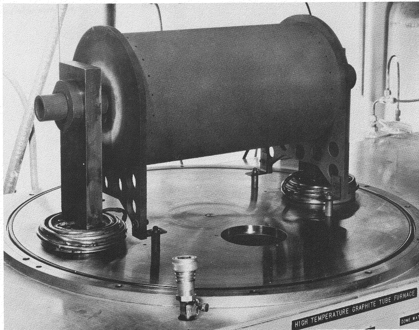
Figure 3 -- King Furnace I with Radiation Shielding in Place.
