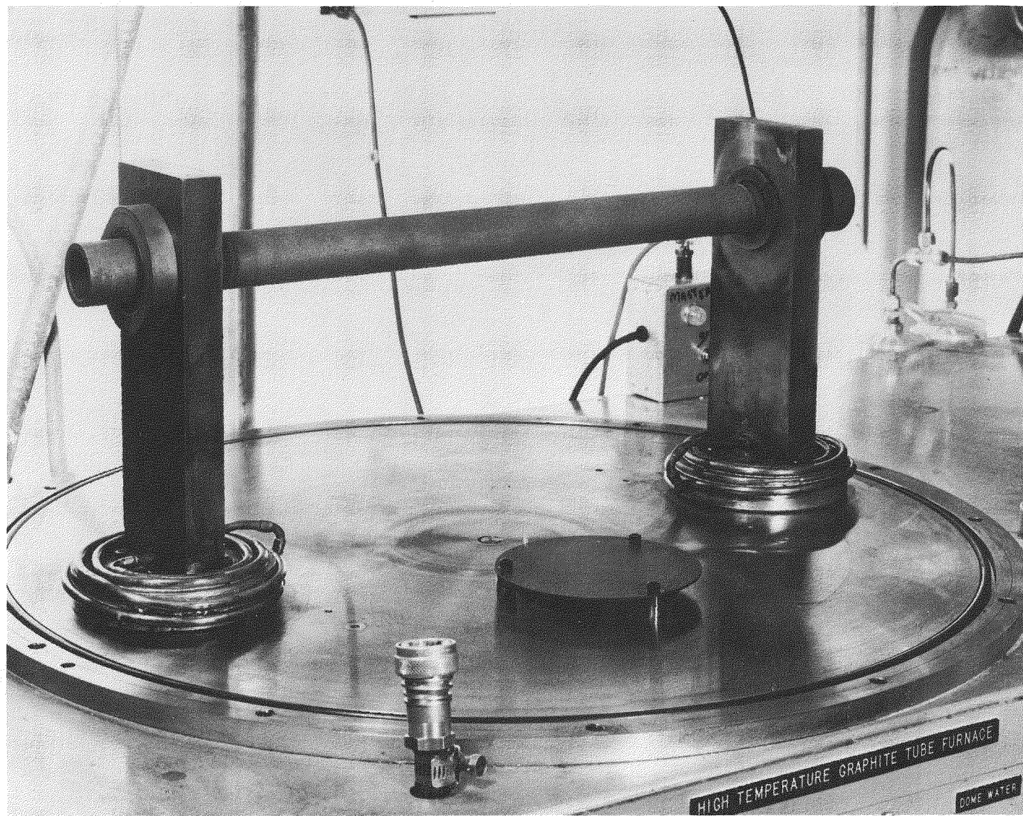
Figure 2 -- King Furnace I with Dome Raised, Showing the Graphite Heating Element (Radiation Shielding Removed).
