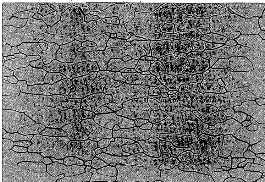
Fig. 2.43 — Photomicrograph of low-carbon (26 ppm) Mo sheet, heat 7722, annealed at 1200°C for 1 hour in vacuum (Neg. 10316, 250X)
