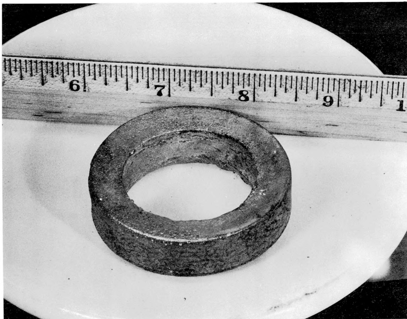
Fig. 6. Plutonium product ring from 500 g. scale experiment - bottom view (No surface cleaning)
