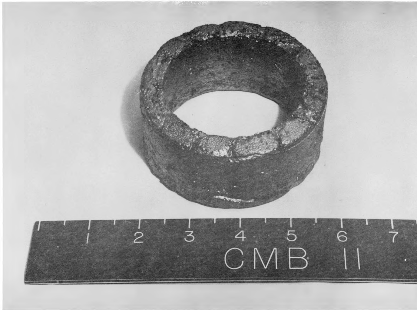
Fig. 12. Plutonium product ring from 3.5 kg. scale experiment - bottom view (No surface cleaning)
