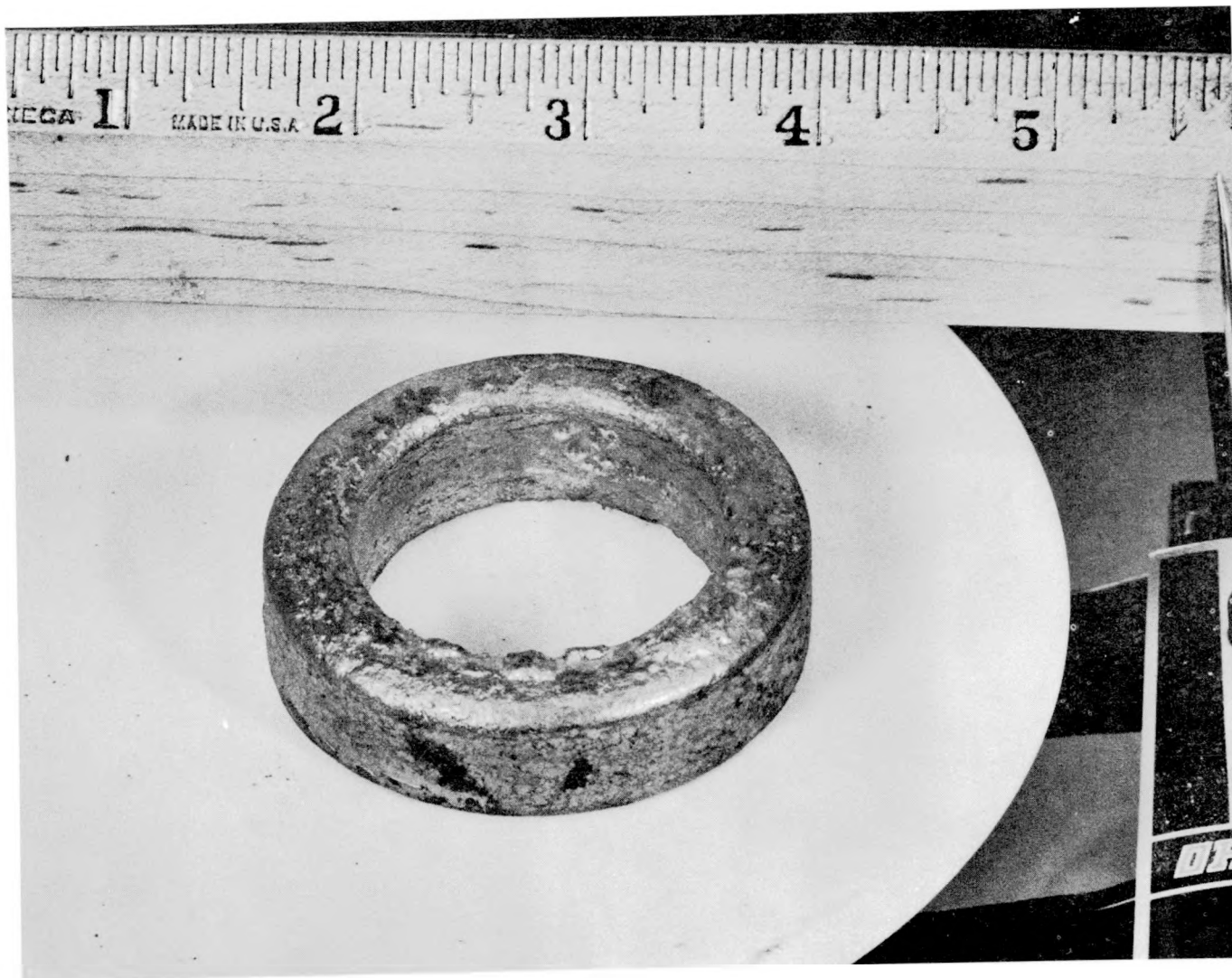
Fig. 5. Plutonium product ring from 500 g. scale experiment - top view (No surface cleaning)
