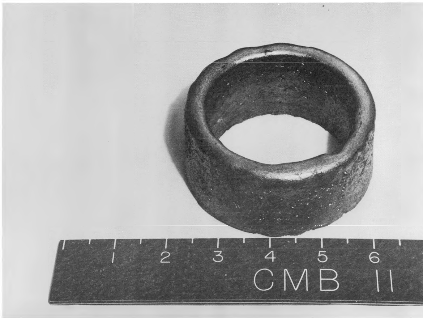
Fig. 11. Plutonium product ring from 3.5 kg. scale experiment - top view (No surface cleaning)
