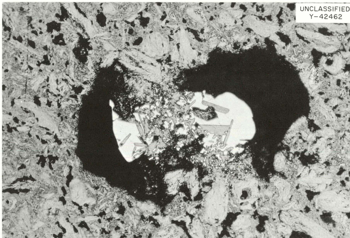
Fig. 11.13. Unirradiated Control Sample of Material from Fuel Pellet b of Capsule MTR-48-2. Note graphite crystals in the UC_2 . Etched. 250X
