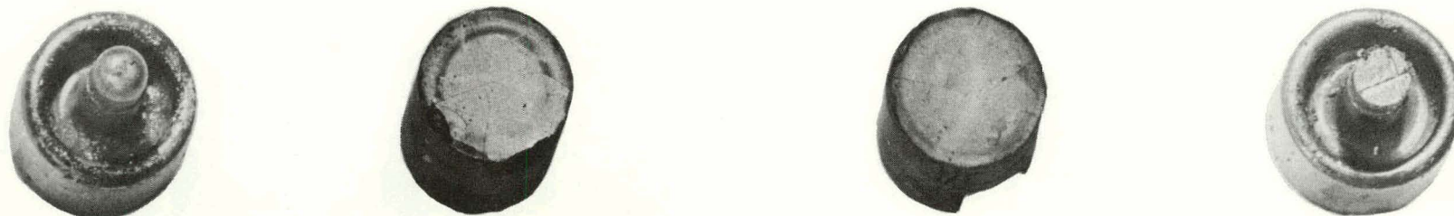
Fig. 12.12. Capsule 04-3, As Opened, Showing Cracked Pellets and End Caps.
