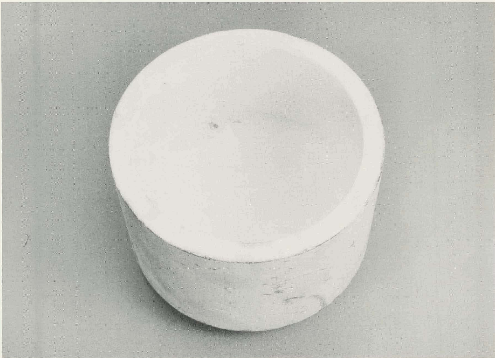
Figure 1. Thoria Coated Graphite Crucibles (6" O.D.)
