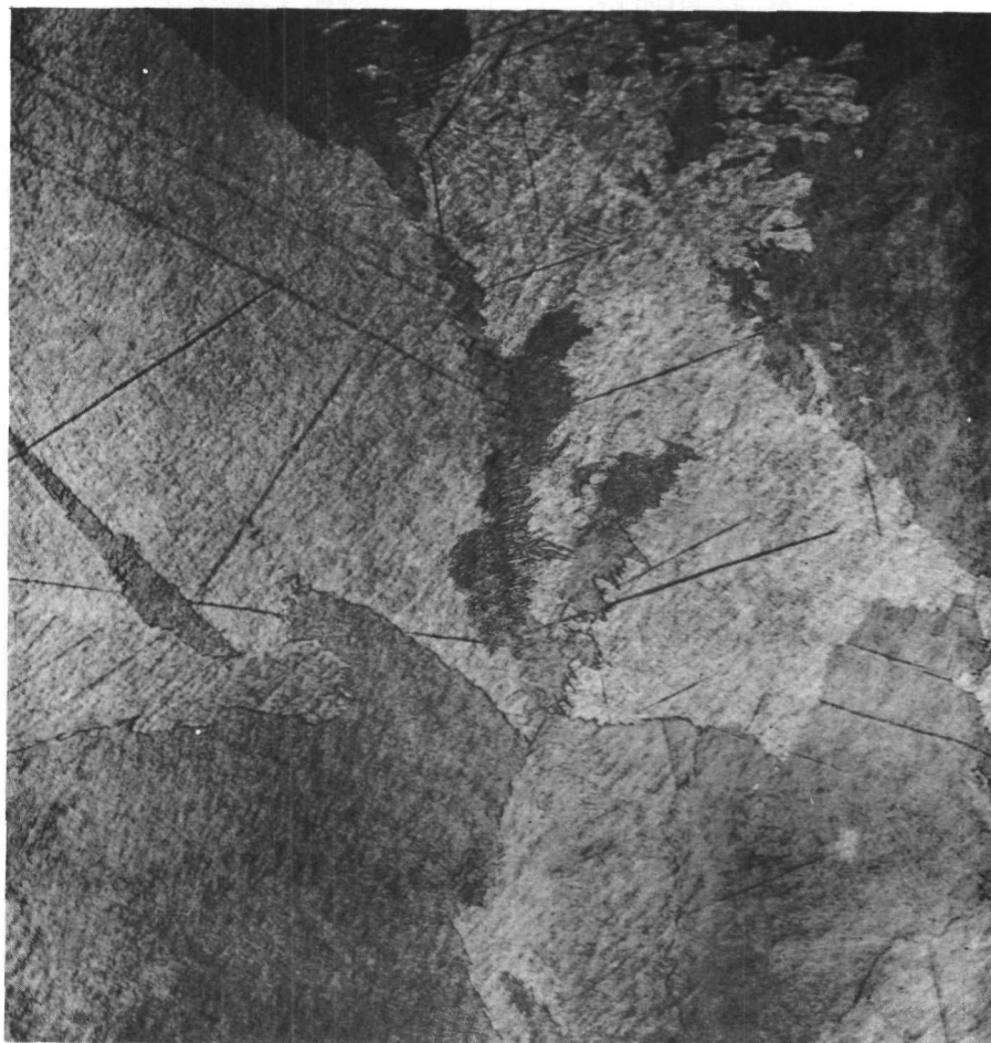
Figure 1. Metallographic structure as revealed by polarized light of zirconium-5 w/o plutonium alloy in the as-cast condition.
