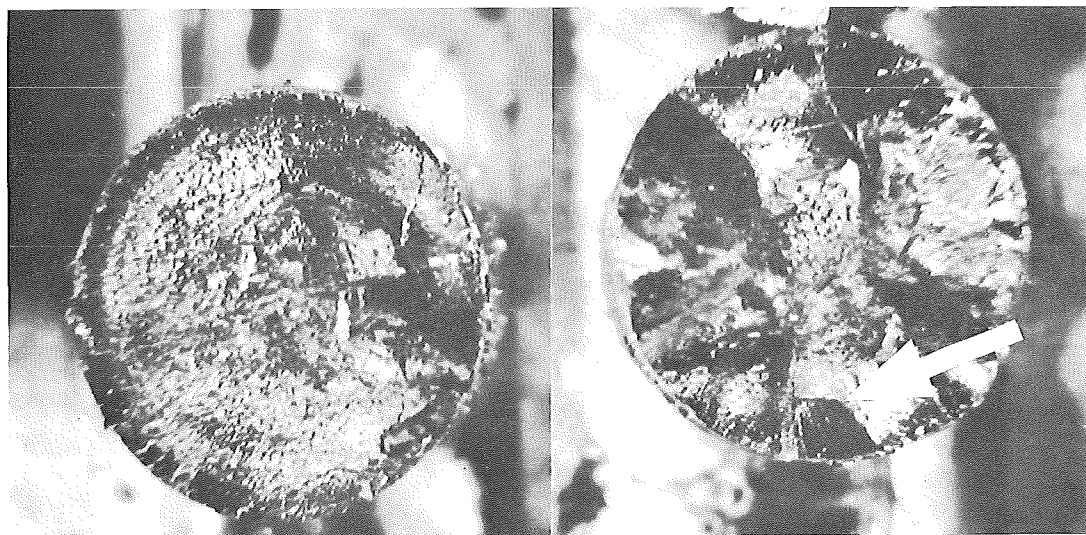
Figure 16 Left photograph cross-section of pellet No. 34 showing organic penetration and slight cracking. Right photograph cross-section of pellet No. 39 with organic penetration 1/3 radius (arrow) and coarse grains at center. Magnification 4X - Reference Nos. 4558 and 4562.
