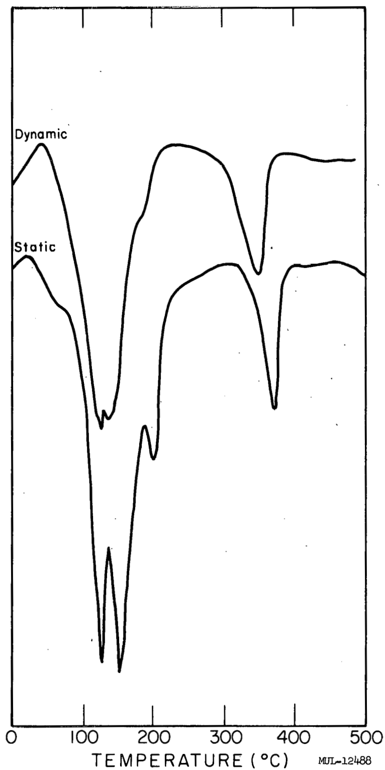
Fig. 3. — Comparison of DTA of \text{La}(\text{C}_2\text{H}_5\text{SO}_4)_3 \cdot 9\text{H}_2\text{O} in static air and dynamic argon atmospheres.
