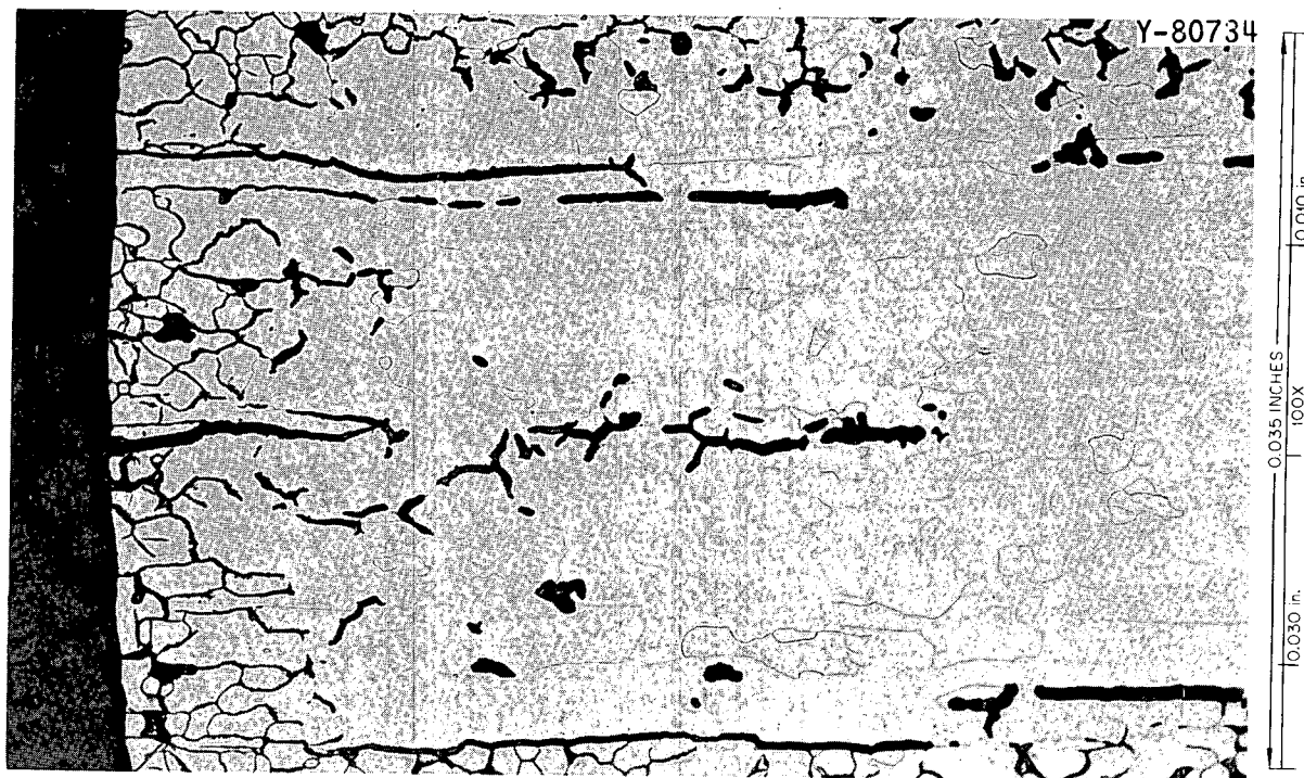
Fig. 5.24. Tantalum, Which Initially Contained 1800 ppm O, After Exposure to Potassium for 100 hr at 800°C. Etched in a solution of H_2O , HNO_3 , and NH_4HF .
