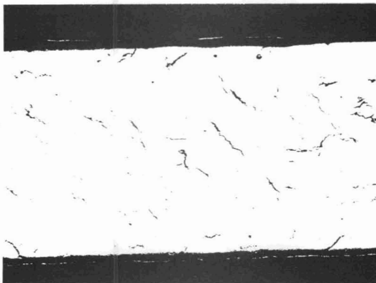
Figure 18. Distribution of hydrides in Zr-Nb heat-affected zone. (Same sample as in Figure 17). Bright Field X 100
