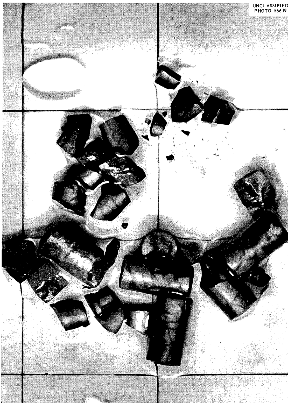
Fig. 4. UO 2 pellets from specimen X-13. Irradiated to 15,150 Mwd/T in NRX reactor. (Background 1" grid.)
