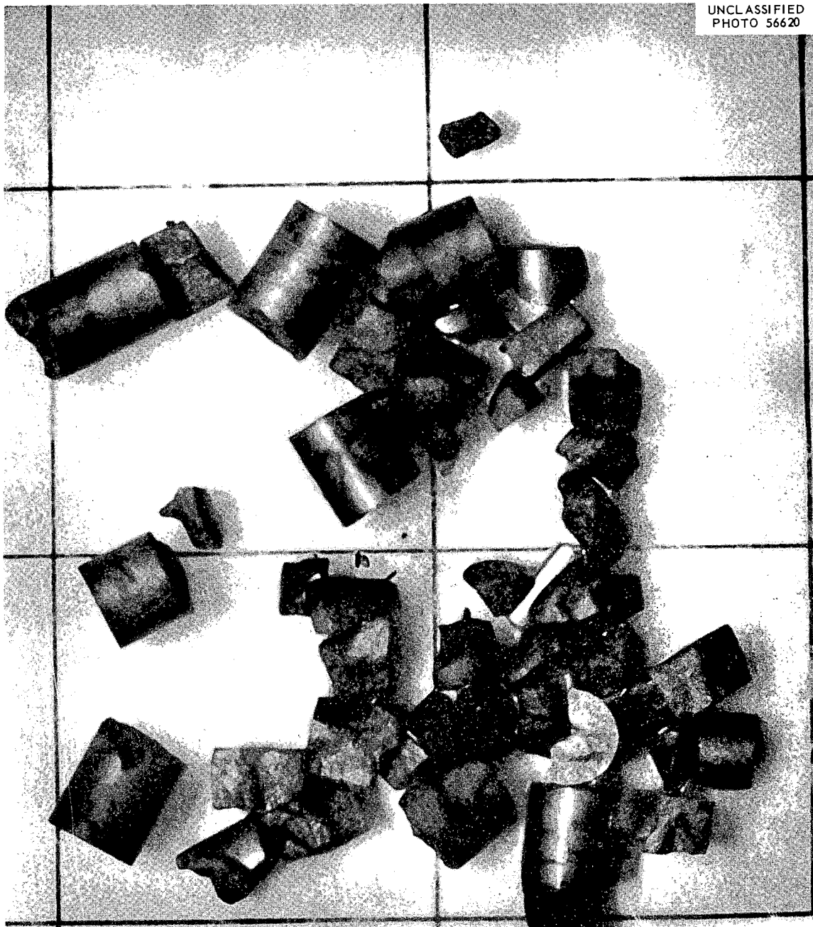
Fig. 5. UO 2 pellets from specimen X-33. Irradiated to 15,150 Mwd/T in NRX reactor. (Background 1" grid.)
