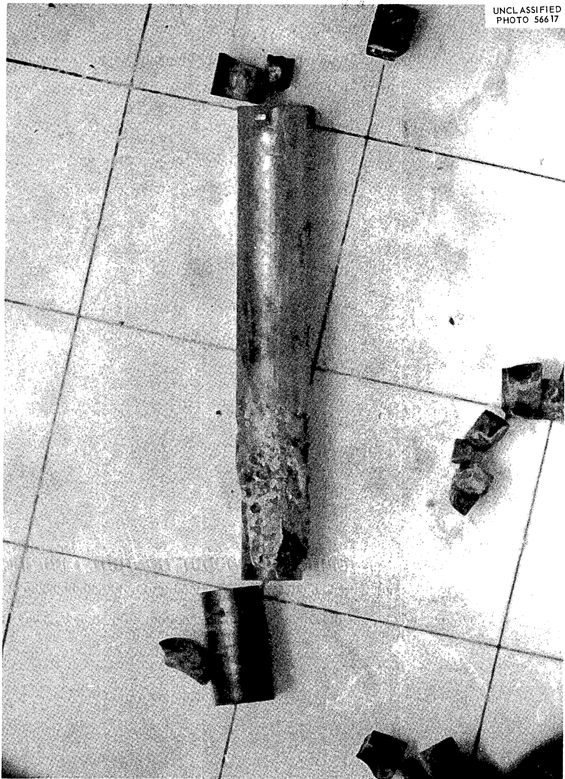
Fig. 2. Zircaloy-2 clad \text{UO}_2 fuel specimen X-33 after 2 hours in boiling 6 \text{M} \text{NH}_4\text{F} - \text{NH}_4\text{NO}_3 . Note the intact \text{UO}_2 pellet. (Background 1" grid.)
