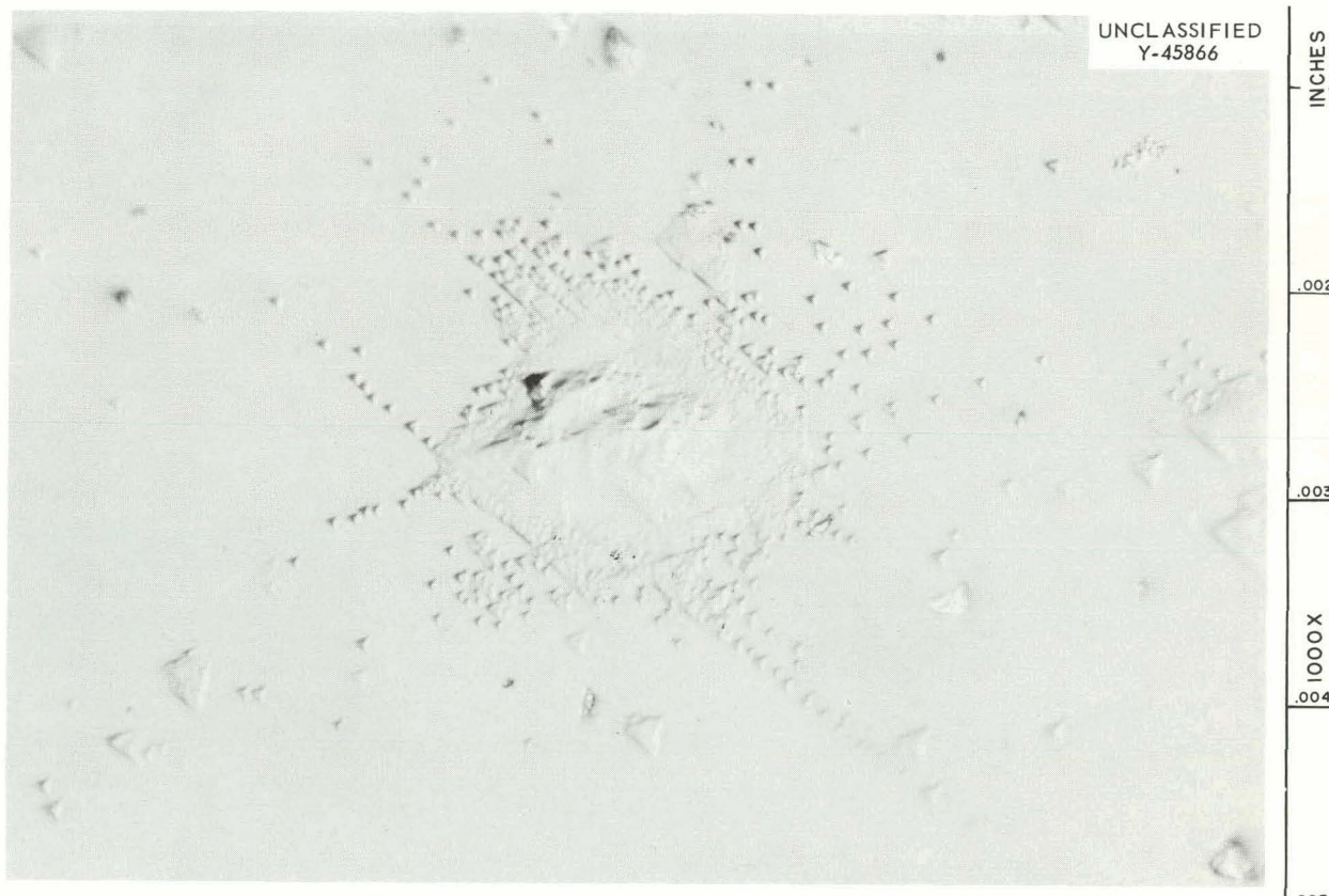
Fig. 24.2. Cleaned Surface of \text{CaF}_2 Single Crystal at Point Where \text{CaF}_2 Particle Had Started To Join Surface. Heated for 30 min at 1200^\circ\text{C} . Sulfamic acid etch. 1000X.
