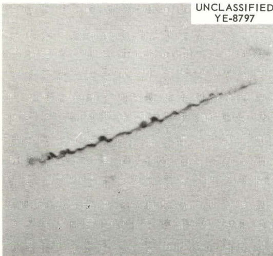
Fig. 28.5. Precipitates at a Dislocation in Niobium Annealed for 1 hr at 900°C. 50,000X.
