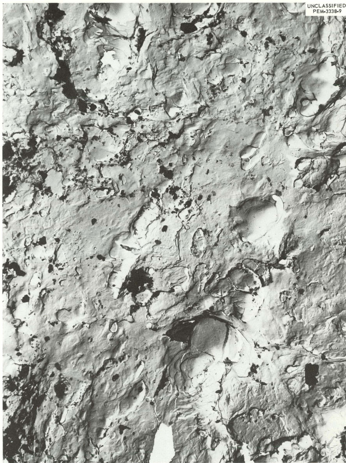
Fig. 22.1. Surface of Irradiated \text{ThO}_2 Pellet Taken at 8000X and Reduced 16%. This electron micrograph was made from a cellulose-acetate replica obtained by remote handling means.
