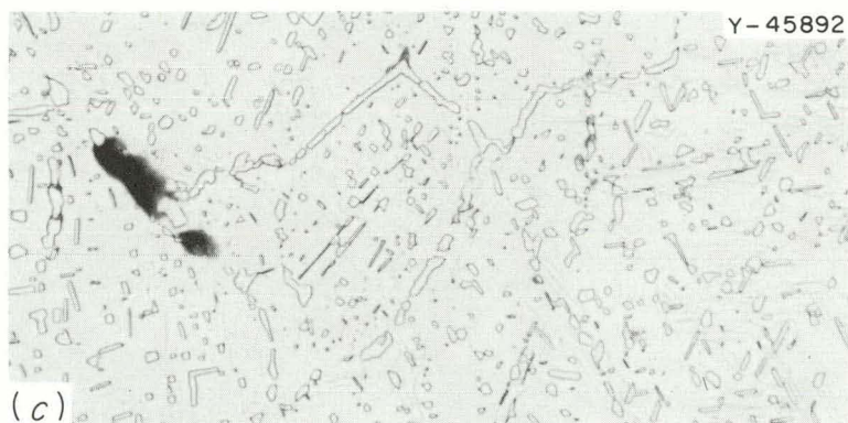
Fig. 14.8. Typical Photomicrographs of Type 304 Stainless Steel Creep-Tested for 5000 hr in Carbon Dioxide at 1500°F. (a) Oxide-oxide interface; (b) oxide-metal interface; (c) metal substrate 0.025 in. from original metal surface. Etchant, aqua regia. 500X. Vendor's analysis of as-received material: 9.55 Ni-18.30 Cr-1.18 Mn-0.07 C (wt %).
