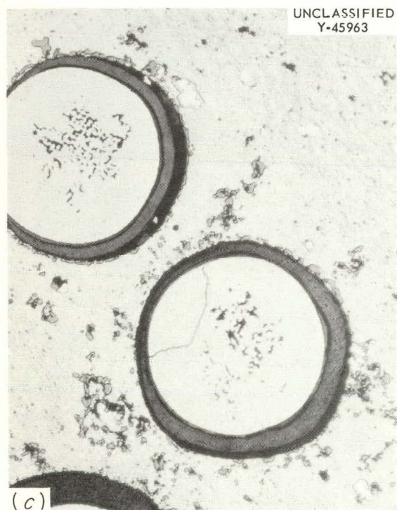
Fig. 19.4. Fissile Particles in a Thorium Matrix Heated at 900^{\circ}\text{C} for 100 hr – (a) Uncoated UC; (b) Niobium-Coated \text{UO}_2 ; (c) Pyrolytic-Carbon-Coated UC; (d) Pyrolytic-Carbon-Coated \text{UC}_2 . Specimens prepared by cold pressing followed by cold swaging. Reaction between dispersoid and matrix is substantial for uncoated UC and niobium-coated \text{UO}_2 (a and b) but is very slight for pyrolytic-carbon-coated UC and \text{UC}_2 (c and d). As-polished. 250X. Reduced 4.5%.
