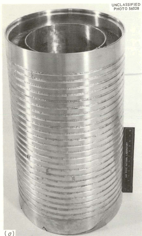
Fig. 21.1. HFIR Flow Test Assembly Showing (a) Circumferential Welded Bands on Element Exterior and (b) Plug Welds on Element Interior.
