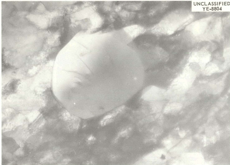
Fig. 28.4. Recrystallized Grain in Niobium Deformed Approximately 95% by Cold Rolling and by Annealing for 1 hr at 600°C. 18,000X.
