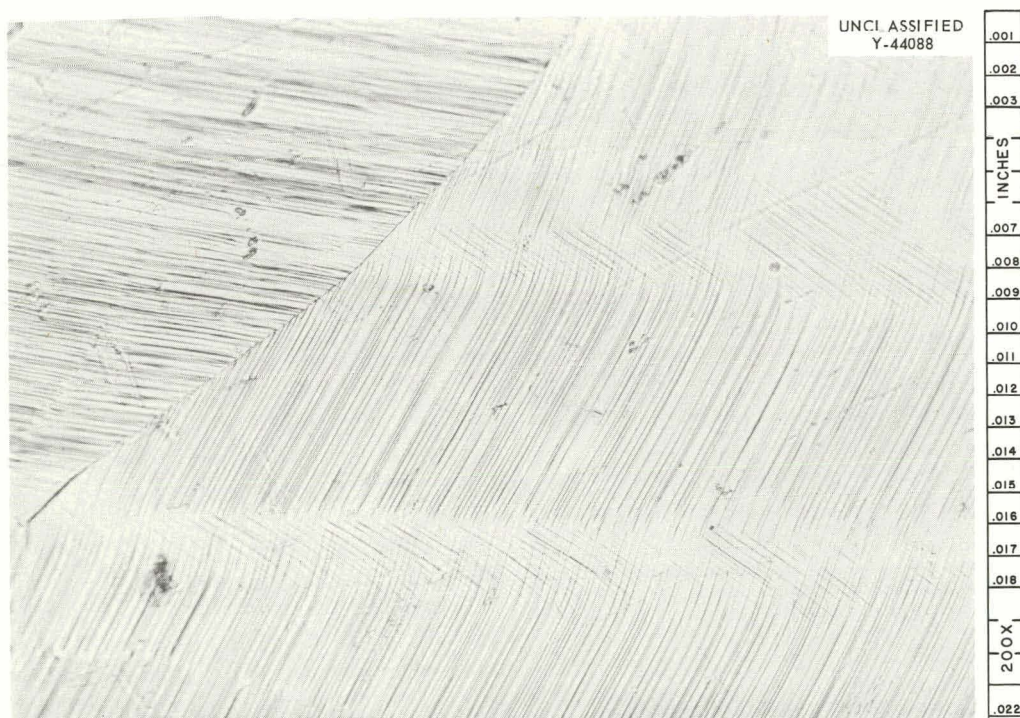
Fig. 33.2. Deformation Bands Caused by Slip on the Primary and Critical Slip Planes in Aluminum. 200X. Reduced 18%.
