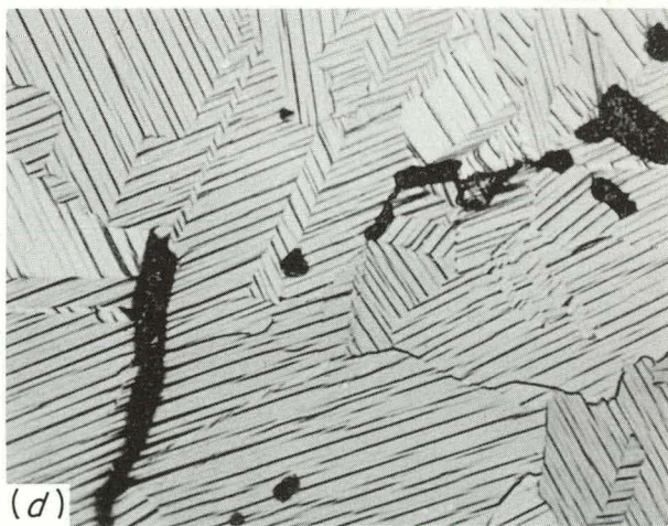
Fig. 28.19. Unusual Etching Behavior of UC Platelets Associated with Shift in UC Lattice Parameter. Etched with 1:1:1 \text{H}_2\text{O} , \text{CH}_3\text{COOH} , \text{HNO}_3 and immersed for 30 sec. 1000X. (a) Gray-type UC platelets; a_0 = 4.948 Å; (b) swelling-type UC platelets; a_0 = 4.963 Å; (c) narrow UC platelets coalescing at flakes of graphite; a_0 = 4.954 Å; (d) normal structure (with flakes of graphite); a_0 = 4.959 Å.
