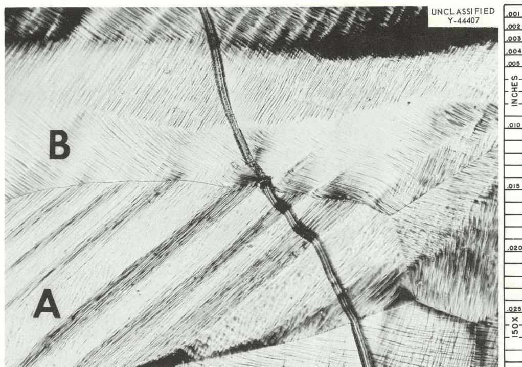
Fig. 33.3. Effects of Grain Boundaries and Neighboring Grains on Deformation of Polycrystalline Aluminum. 150X. Reduced 18%.
