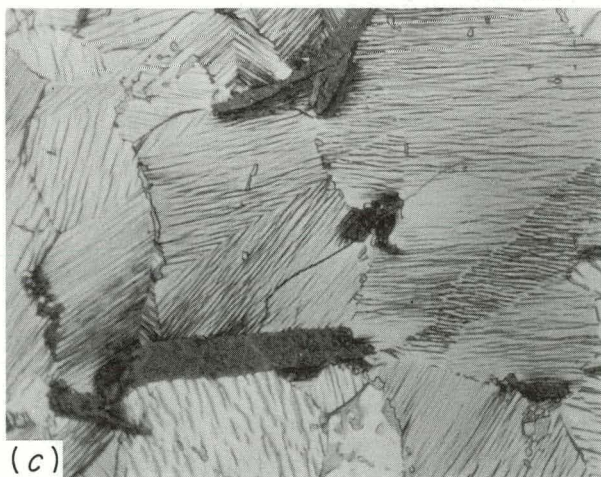
Fig. 28.19. Unusual Etching Behavior of UC Platelets Associated with Shift in UC Lattice Parameter. Etched with 1:1:1 \text{H}_2\text{O} , \text{CH}_3\text{COOH} , \text{HNO}_3 and immersed for 30 sec. 1000X. (a) Gray-type UC platelets; a_0 = 4.948 Å; (b) swelling-type UC platelets; a_0 = 4.963 Å; (c) narrow UC platelets coalescing at flakes of graphite; a_0 = 4.954 Å; (d) normal structure (with flakes of graphite); a_0 = 4.959 Å.
