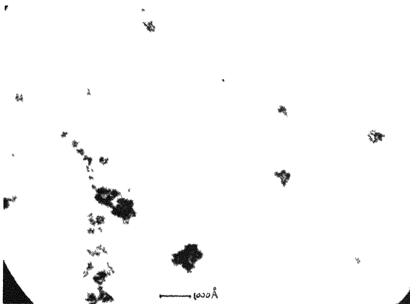
FIG.7. 1 M PuO 2 sol with UO 3 /Pu ratio of 0.2, diluted 10 000 times with water.
