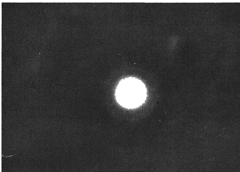
FIG.9. Typical electron diffraction image, similar in all \text{PuO}_2 sols.
