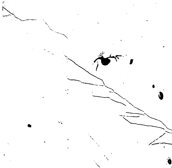
a. Veined martensitic alpha. Etchant: Phosphoric Acid. Micro No. 14808.
