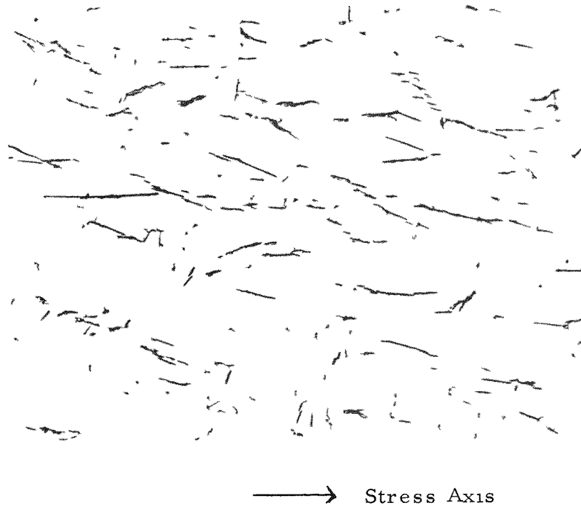
Figure 12 (Met. E13-62) Hydride Orientation in Hydrided Specimens.
