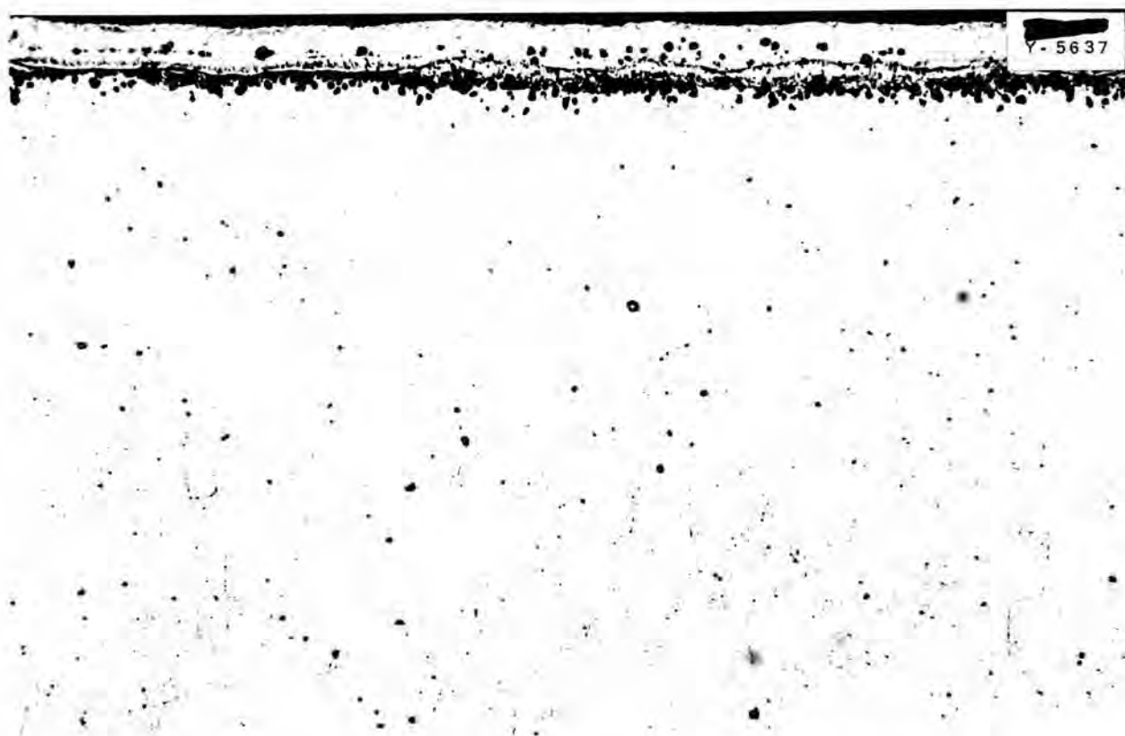
Fig. 32. Corrosion of Inconel in a Fluoride Fuel [(\text{NaF-KF-UF}_4) + 2\% \text{ Zr}] for 100 hr at 816^\circ\text{C} . 200X.
