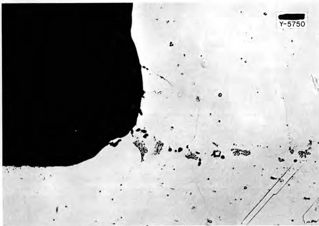
Fig. 44. Corrosion Test of Microbrazed Inconel Tube-to-Header Joint Exposed to \text{NaF-KF-LiF-UF}_4 for 100 hr at 1500^\circ\text{F} . 250X.
