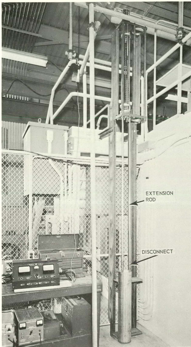
Fig. 11-4 - Actuator test stand (Neg. 4268-4)
