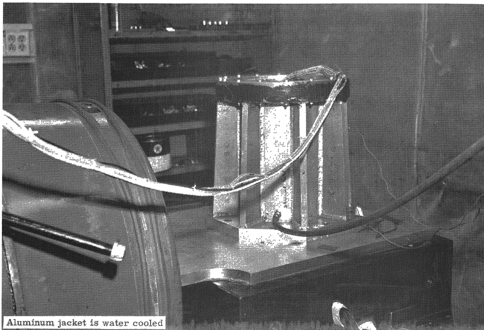
Fig. IX-7. SNAP 7A-7C Thermoelectric Generator and Test Fixture Positioned on Vibration Slide Table for Horizontal Excitation
